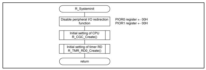
Figure 4.4 Initial Setting of Peripheral Functions
