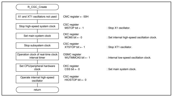
Figure 4.5 Initial Setting of the CPU
