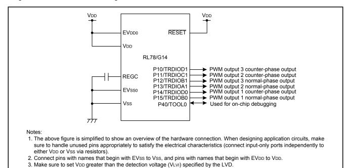
Figure 3.1 Hardware Configuration
