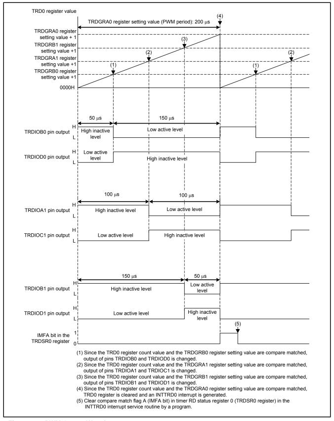
Figure 4.1 PWM Output Waveform
