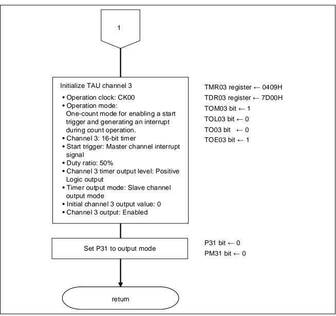
Figure 5.10 Timer Array Unit Setup (2/2)
