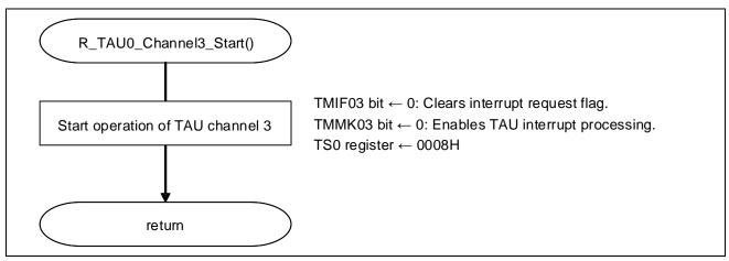
Figure 4.11 Timer Array Unit 0 Operation Start
