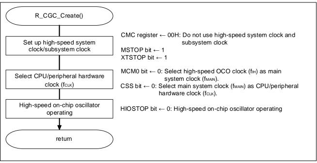
Figure 4.7 CPU Clock Setup
