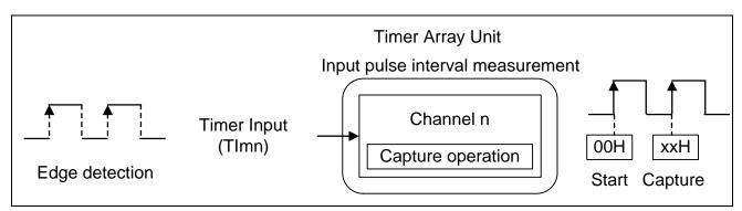
Figure 4.1 Operation Overview (Example of Migration from Input Capture Mode)
