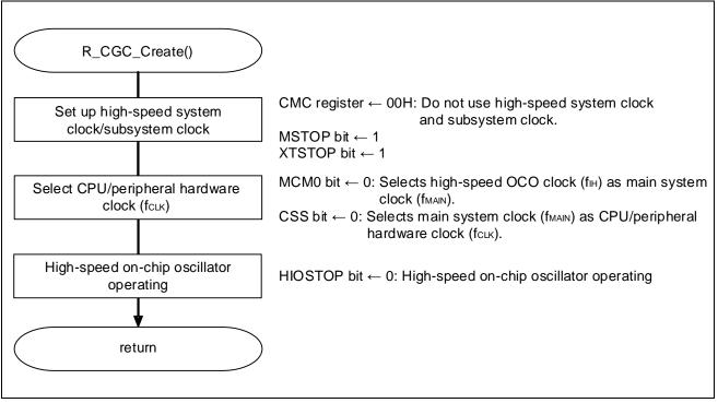
Figure 5.7 CPU Clock Setup
