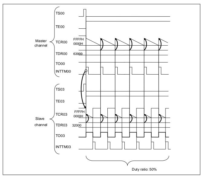
Figure 5.3 Overview of Timer Operation and Interrupts
