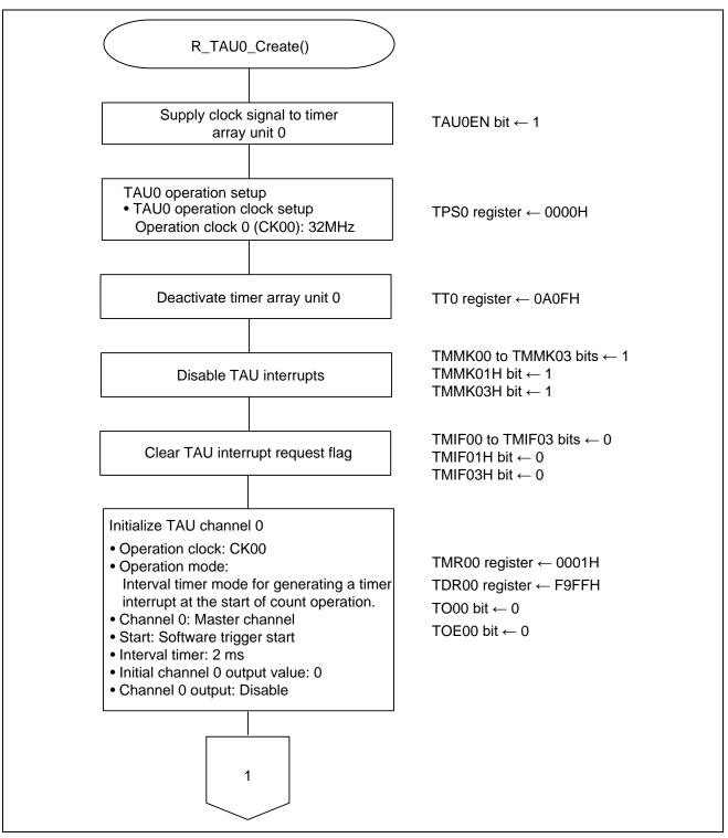
Figure 5.9 Timer Array Unit Setup (1/2)
