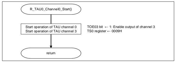
Figure 5.12 Timer Array Unit Startup
