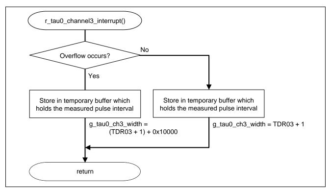
Figure 4.12 INTTM03 Interrupt Processing
