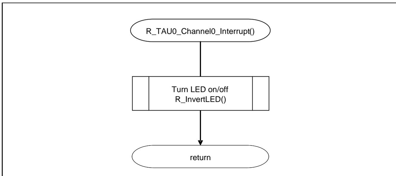
Figure 5.11 INTTM00 Interrupt Processing
