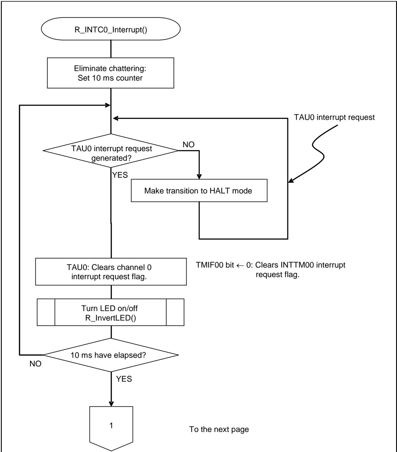
Figure 5.13 INTPO Interrupt Processing (1/2)
