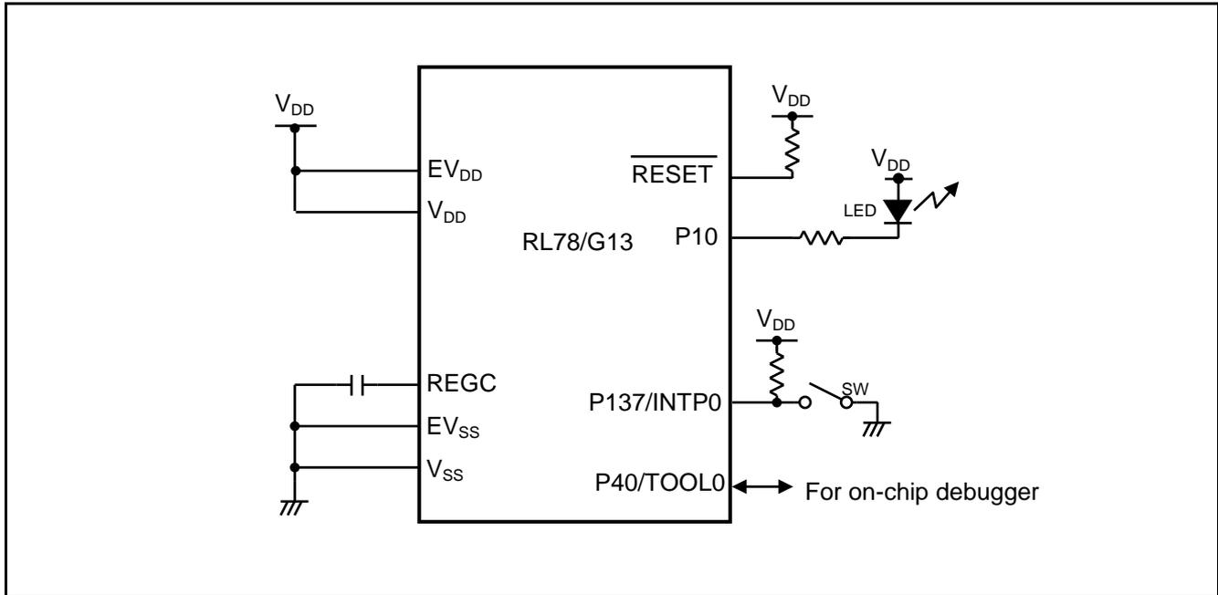
Figure 4.1 Hardware Configuration
