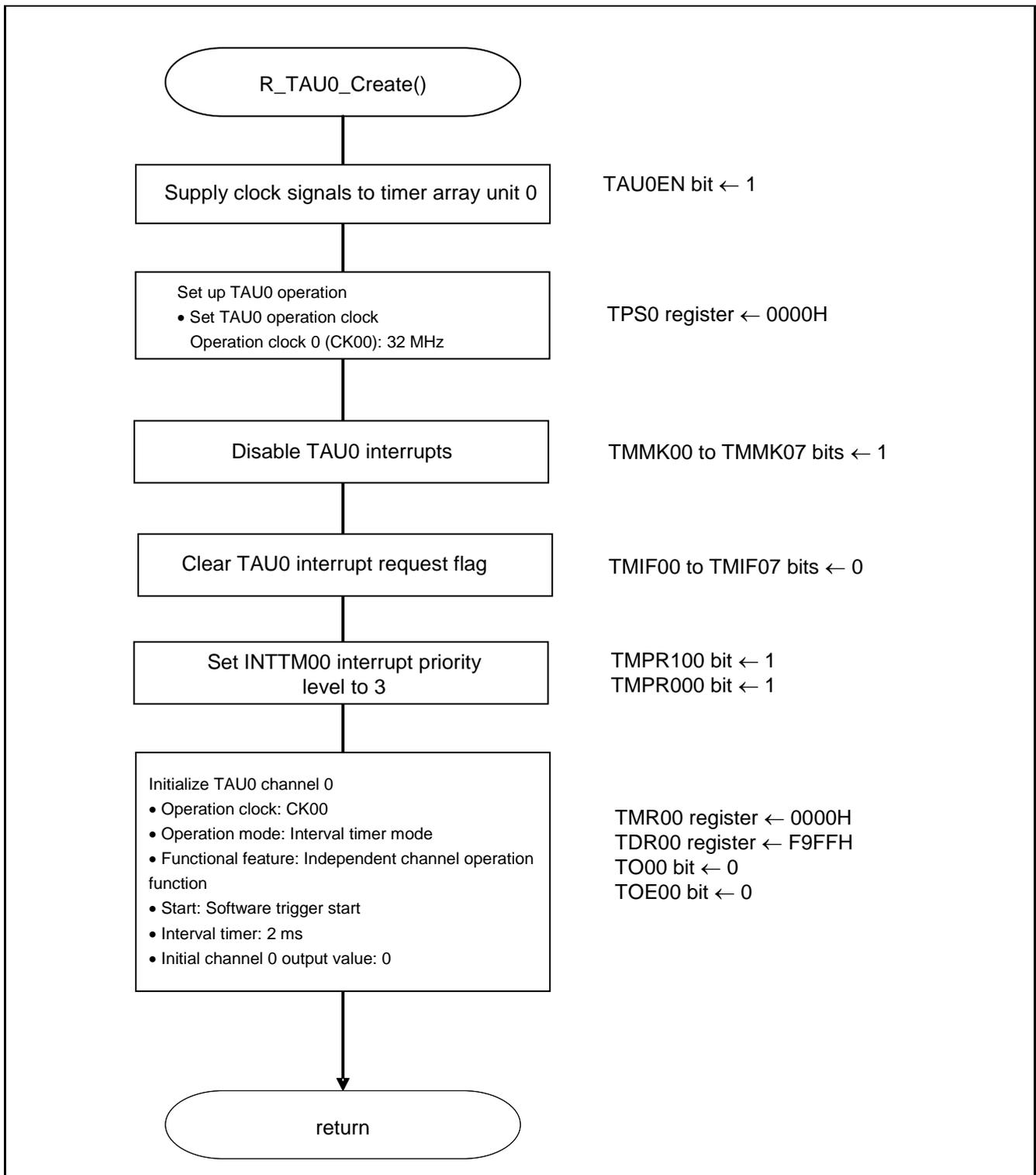
Figure 5.6 Timer Array Unit Setup
