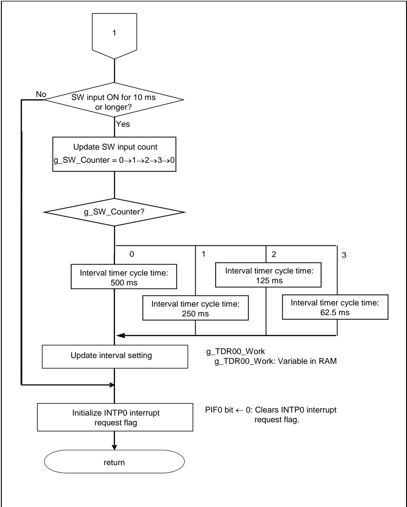
Figure 5.14 INTP0 Interrupt Processing (2/2)
