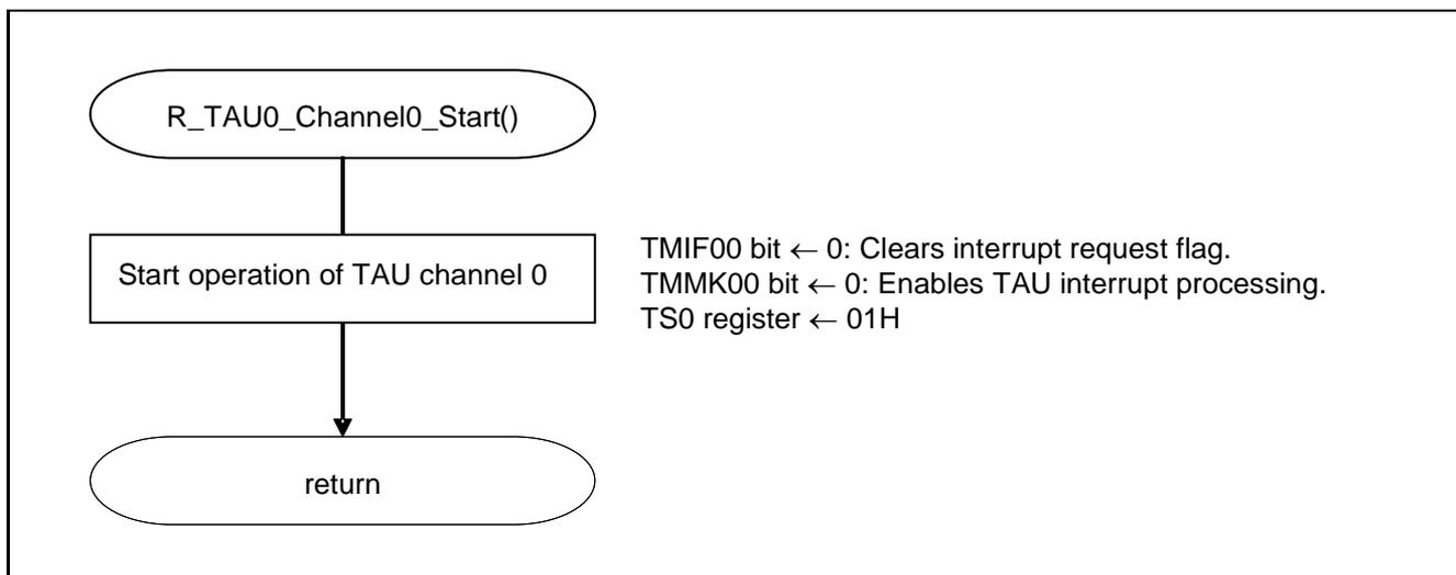
Figure 5.10 Timer Array Unit 0 Operation Start
