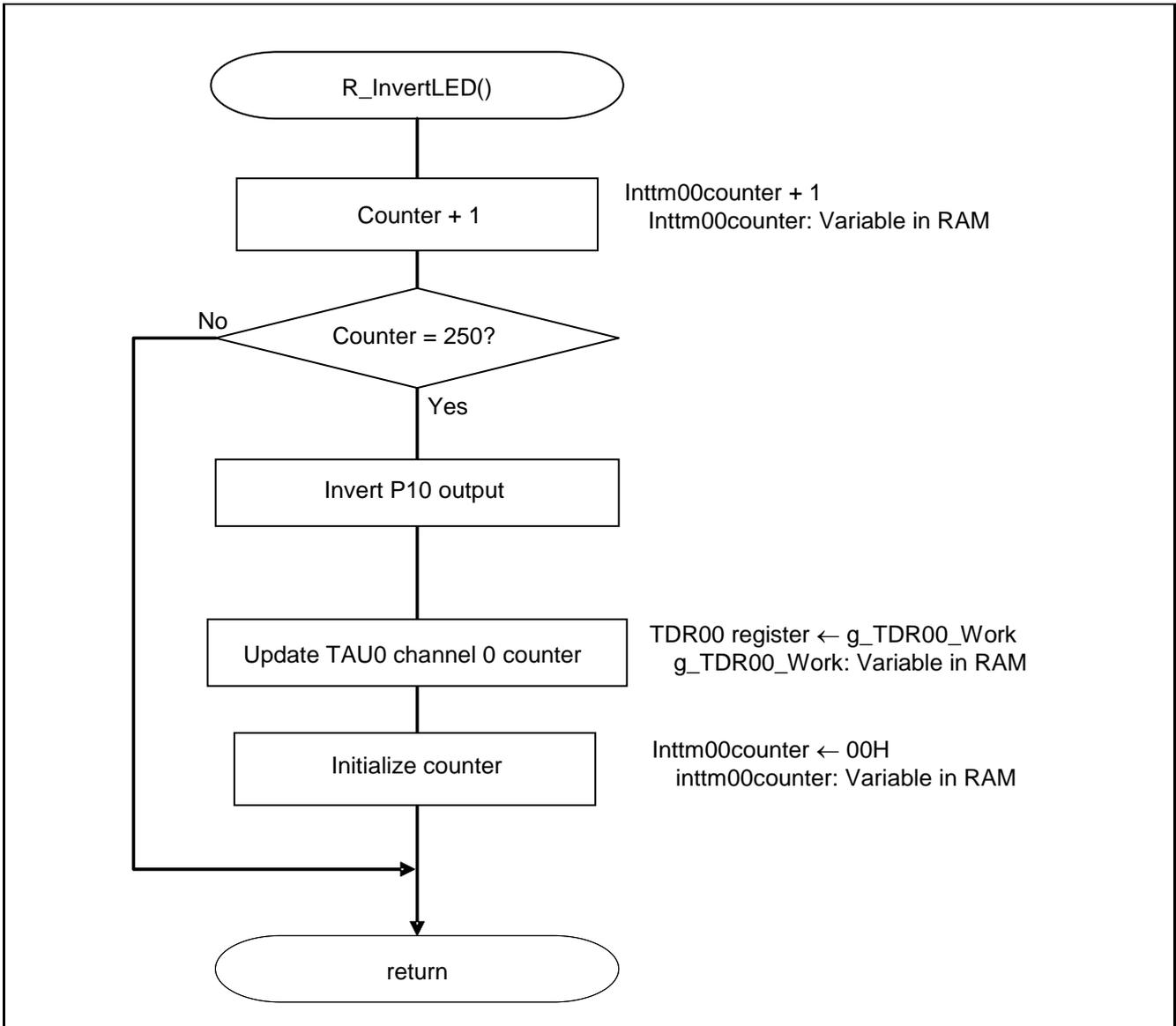
Figure 5.12 Checking Whether 500 ms Have Elapsed
