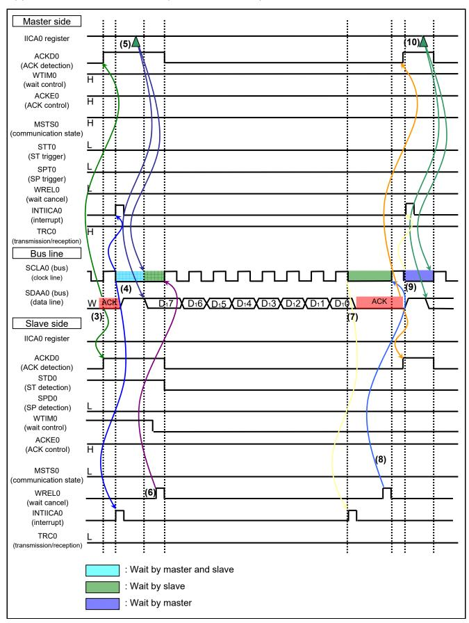
Figure 1.3 IIC Communication Timing Chart (Master-to-Slave Communication Example) (2/4)
