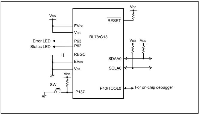
Figure 4.1 Hardware Configuration
