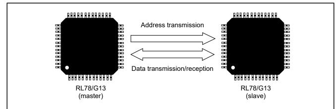
Address transmission: Each device connected to an IIC bus has a unique address. The master transmits a slave address for transmission. The address (7 bits) and the transfer direction (1 bit) are transmitted as one data byte. After receiving the one byte of data, the slave generates an acknowledge signal. Data transmission/reception: Operation, after address reception, to transmit data to the master or to receive data from the master.
