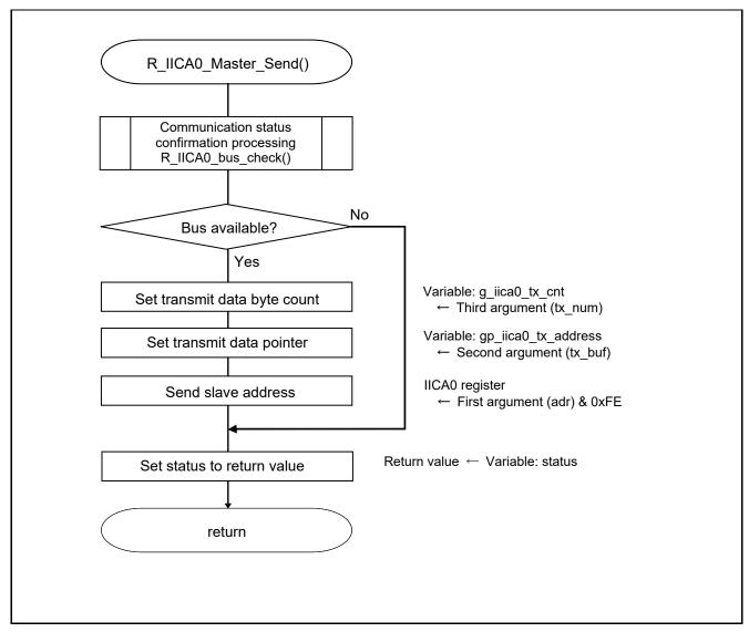
Figure 5.20 Master Transmission Start Request Processing
