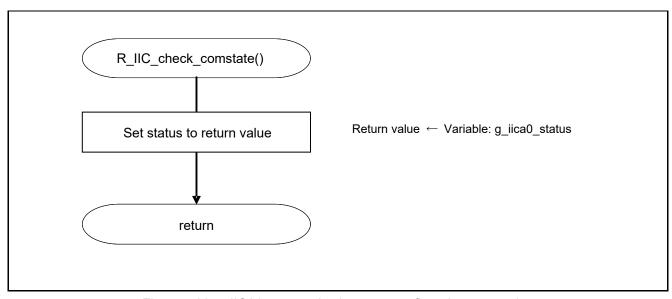
Figure 5.22 IICA0 communication state confirmation processing
