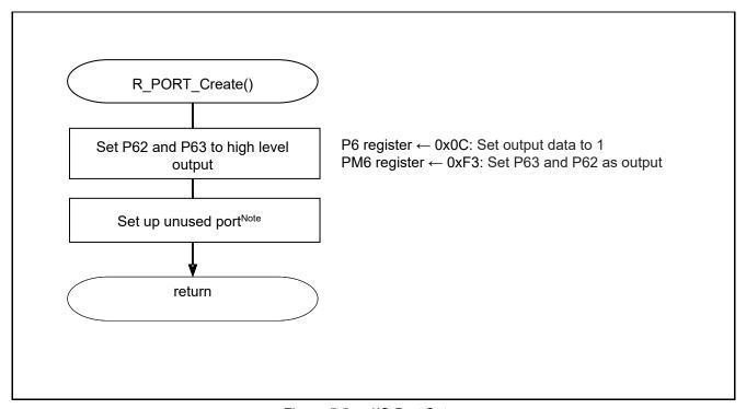
Figure 5.5 I/O Port Setup
