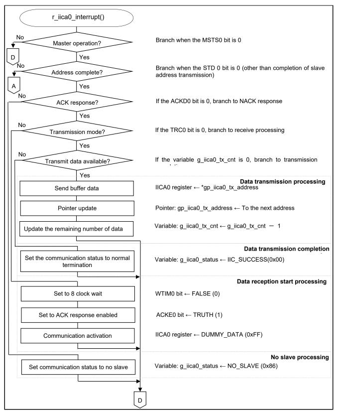
Figure 5.26 IICA0 Interrupt Processing (1/3)
