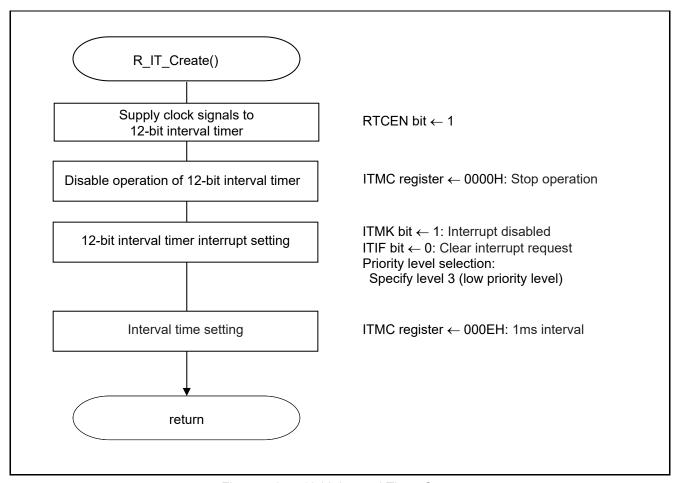
Figure 5.8 12-bit Interval Timer Setup
