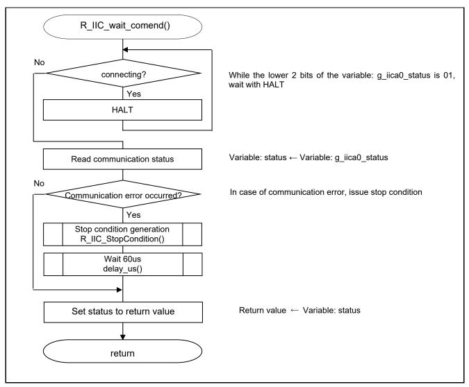
Figure 5.23 Communication completion wait processing
