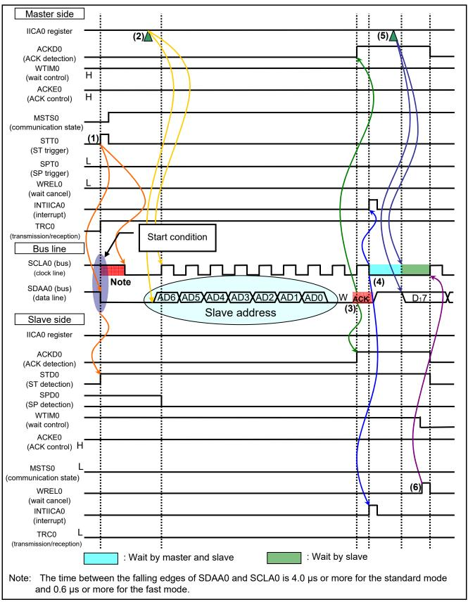
Figure 1.2 IIC Communication Timing Chart (Master-to-Slave Communication Example) (1/4)
