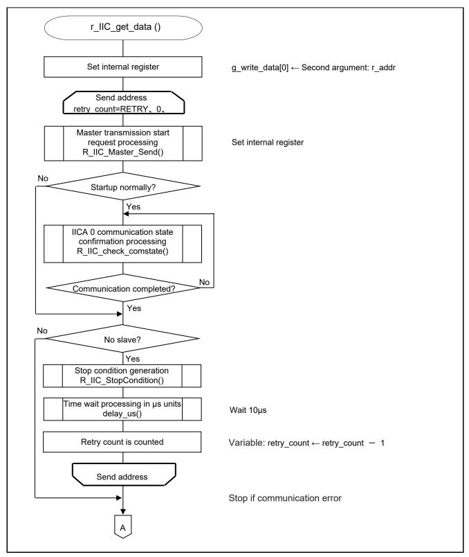
Figure 5.18 processing to receive data from slave (1/2)
