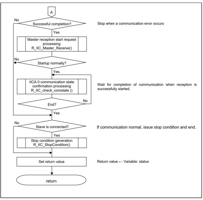
Figure 5.19 processing to receive data from slave (2/2)
