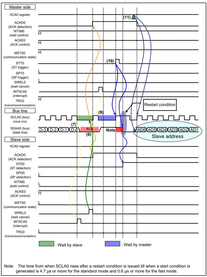
Figure 1.5 IIC Communication Timing Chart (Master-to-Slave Communication Example) (4/4)
