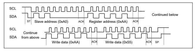
Figure. 1.12 Timing Chart for Continuous Data Writing by Register Address Specification
