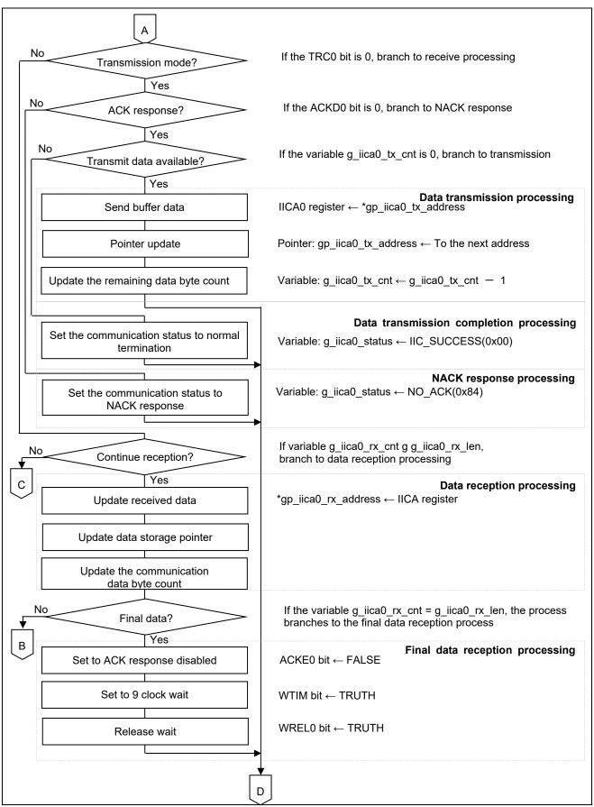
Figure 5.27 IICA0 Interrupt Processing (2/3)
