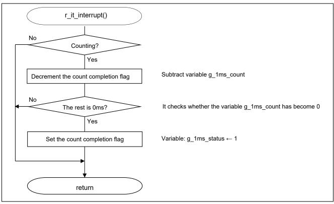
Figure 5.15 12-bit interval timer interrupt processing
