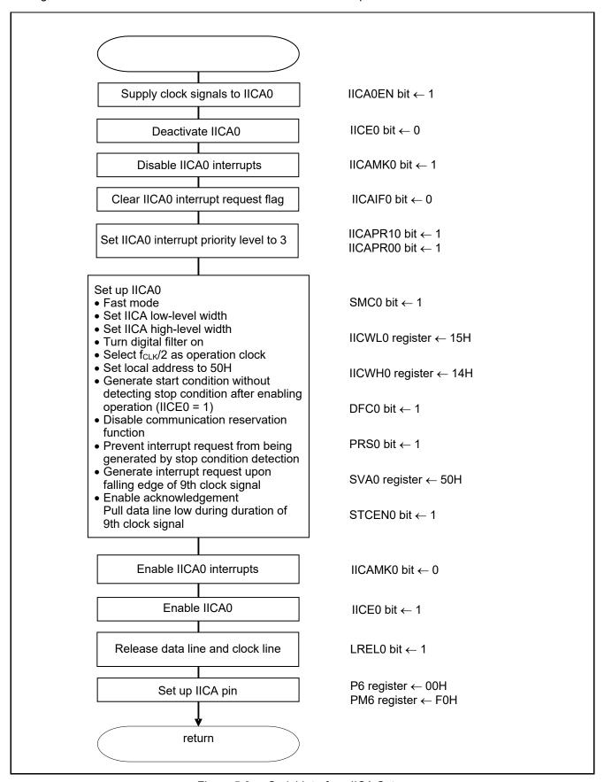
Figure 5.6 Serial Interface IICA Setup
