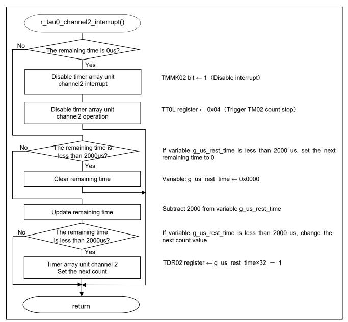
Figure 5.31 Timer Array Unit Channel2 Interrupt Processing
