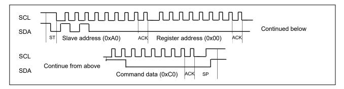
Figure. 1.10 Command Setting Timing Chart
