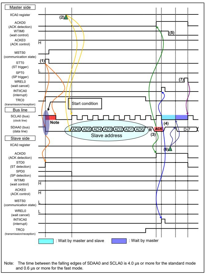
Figure 1.6 IIC Communication Timing Chart (Slave-to-Master Communication Example) (1/3)
