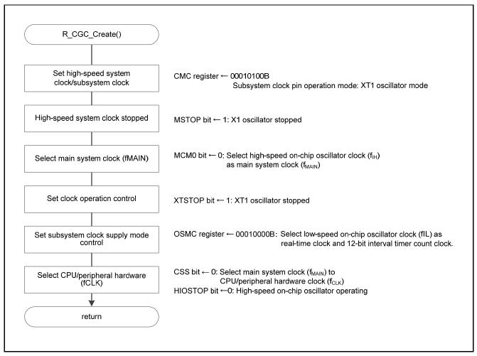
Figure 5.4 CPU Clock Setup
