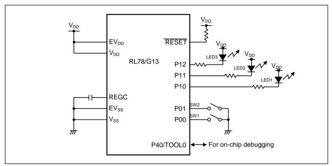
Figure 3.1 Hardware Configuration
