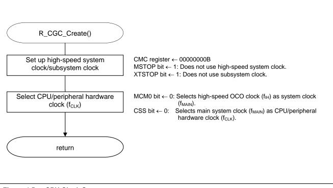
Figure 4.5 CPU Clock Setup
