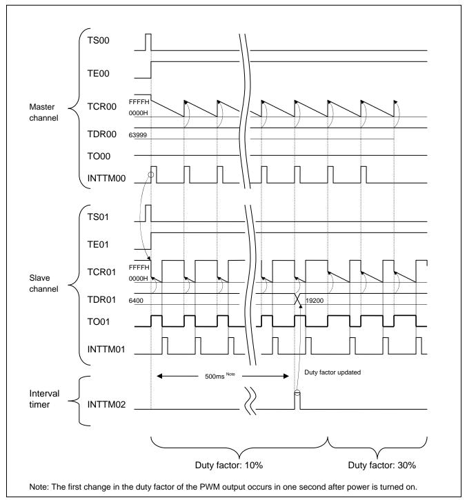
Figure 1.2 Timing Chart which Outlines PWM Output Operation
