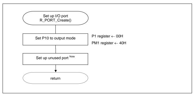
Figure 5.4 I/O Port Setup
