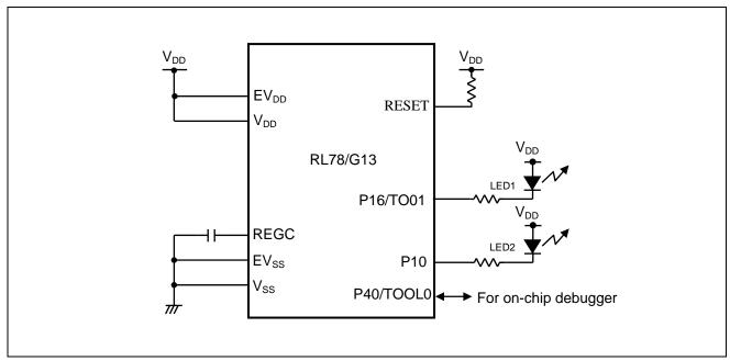
Figure 4.1 Hardware Configuration
