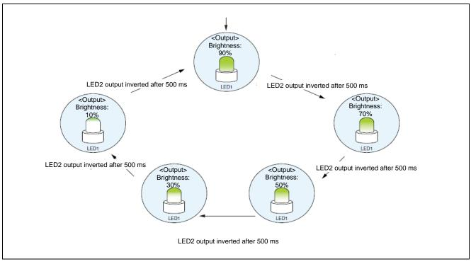
Figure 1.1 Overview of PWM Output Operation
