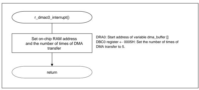
Figure 5.14 DMA Transfer End Interrupt Processing
