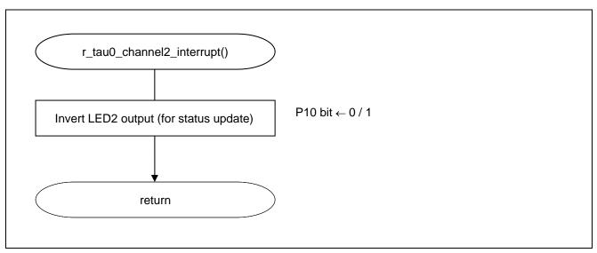
Figure 5.13 TAU0 Timer Interrupt Processing (Channel 2)
