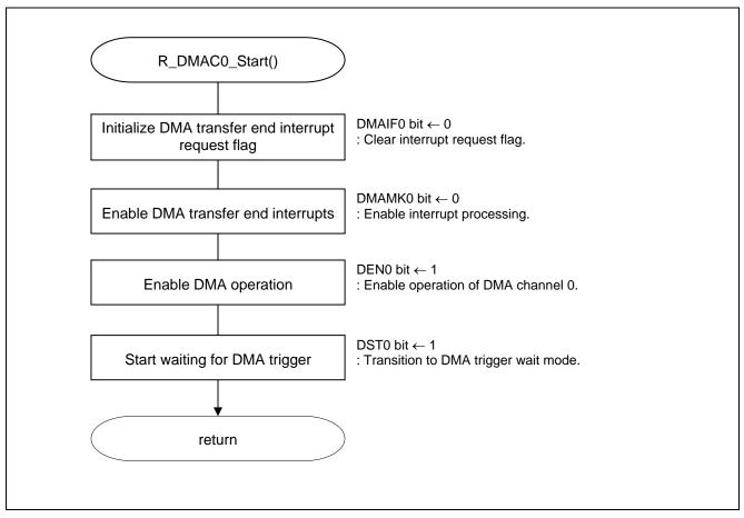
Figure 5.11 DMA Transfer Enable Processing
