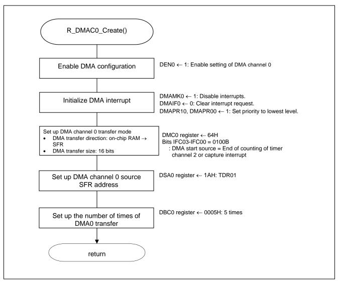
Figure 5.8 Initializing DMA Controller
