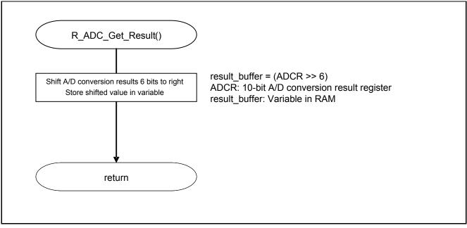
Figure 5.10 Storing the A/D Conversion Results in RAM
