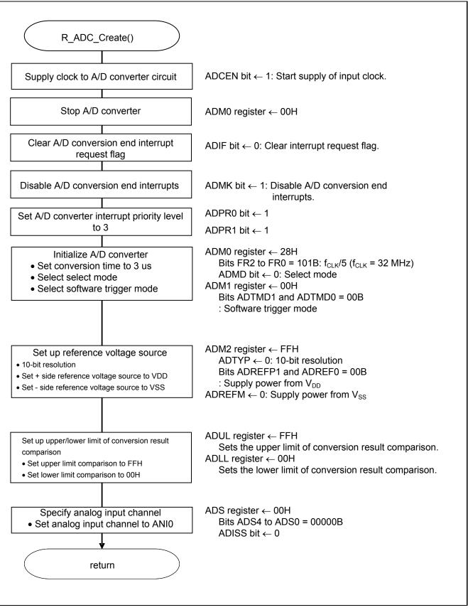
Figure 5.6 A/D Converter Setup Flowchart
