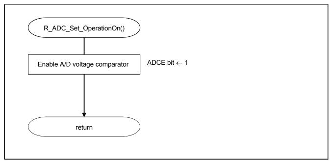
Figure 5.8 Enabling the A/D Voltage Comparator
