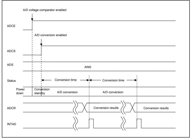
Figure 1.1 Outline of the A/D Converter Conversion Processing
