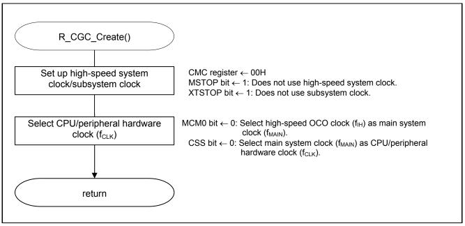
Figure 5.5 CPU Clock Setup
