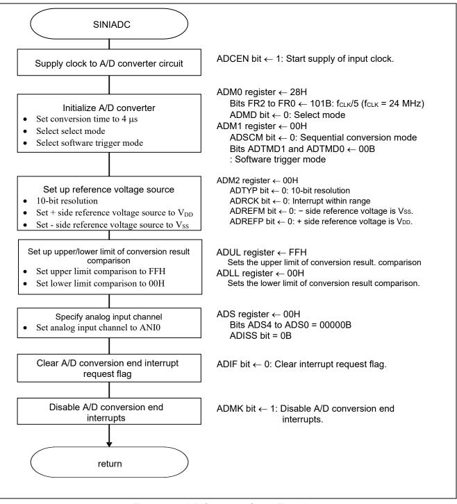
Figure 5.5 A/D Converter Setup Flowchart
