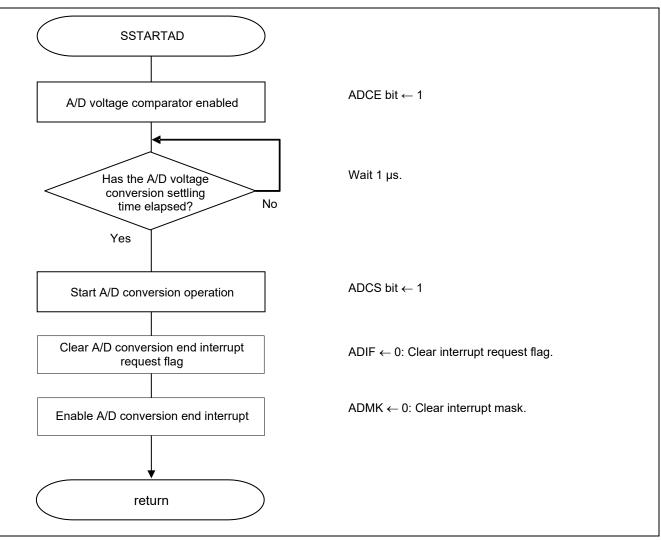
Figure 5.7 A/D Conversion Start Processing
