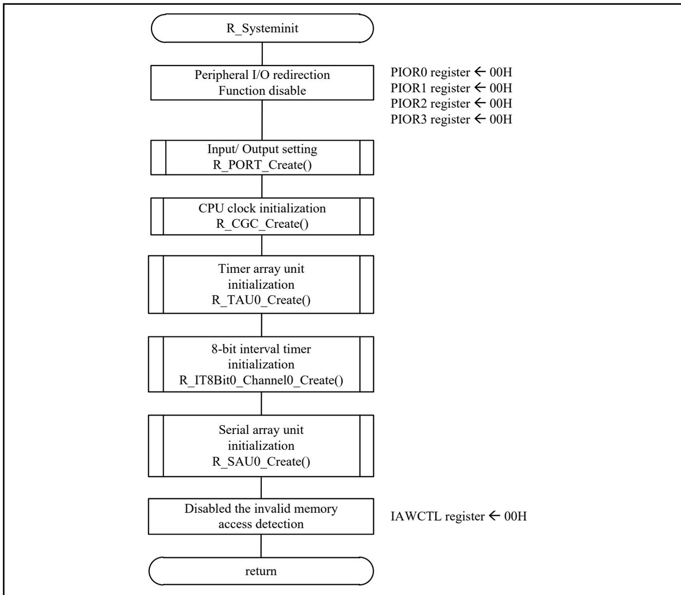
Figure 5.5 Peripheral function initialization function
