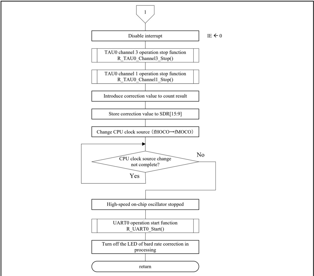
Figure 5.23 8-bit interval timer interrupt function (2/2)
