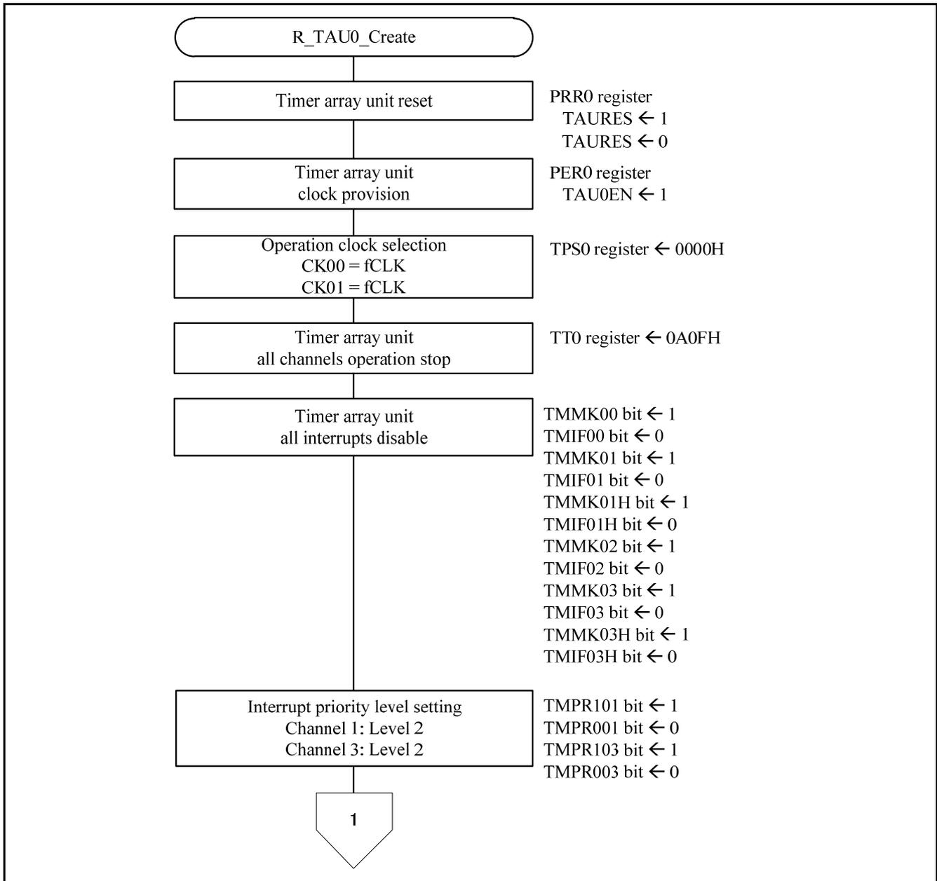
Figure 5.8 Timer array unit initialization(1/2)
