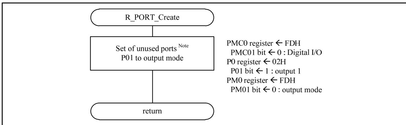
Figure 5.6 I/O Port Setup
