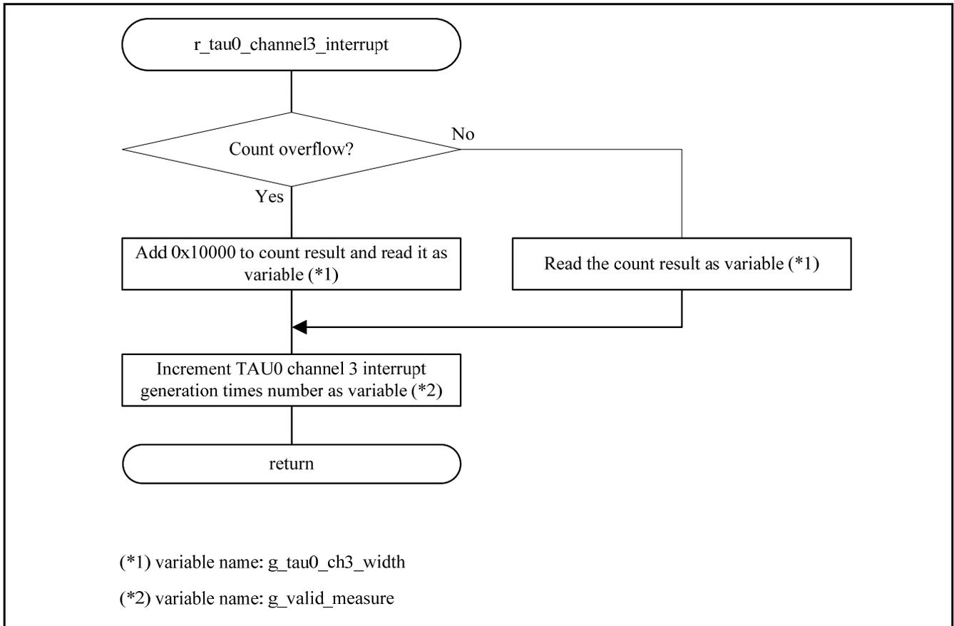
Figure 5.24 TAU channel 3 count complete interrupt function
