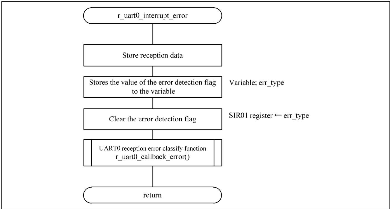
Figure 5.20 UART0 reception error interrupt function
