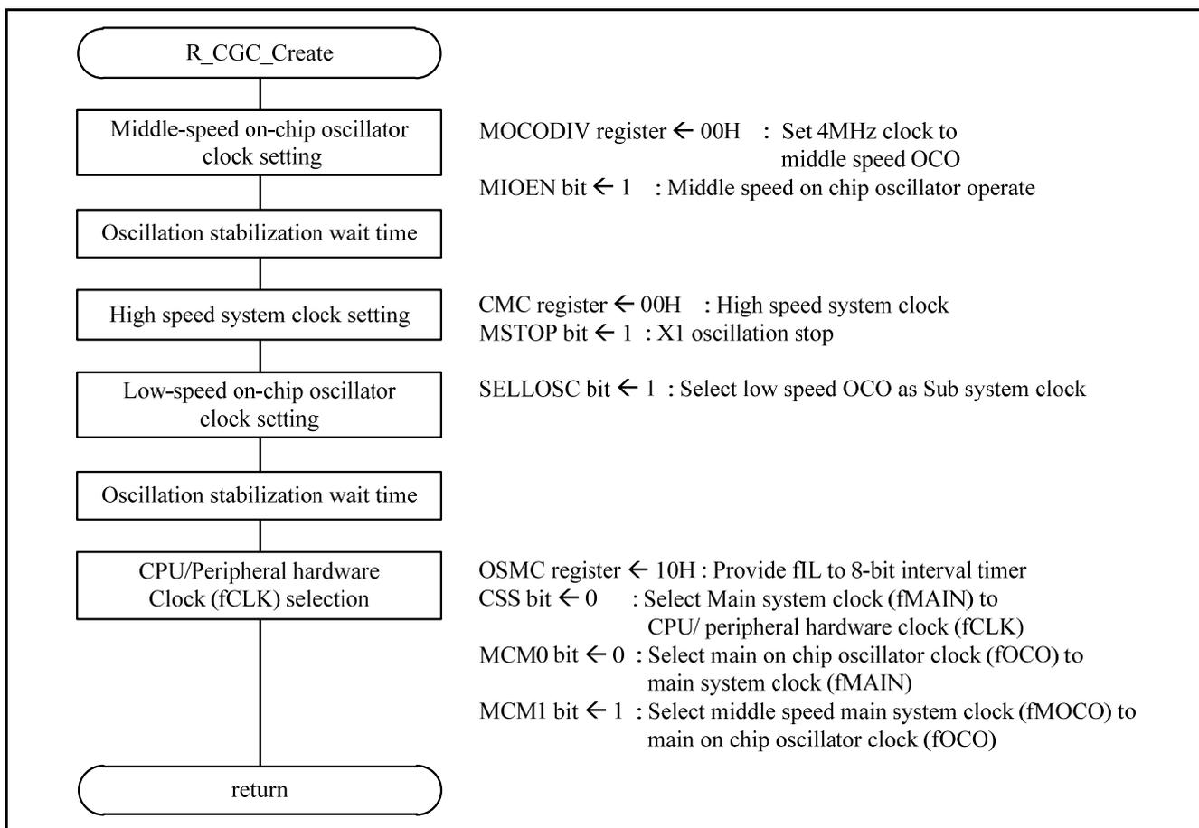
Figure 5.7 CPU clock initialization function
