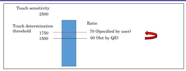
Figure 3 Example of changing the threshold ratio
