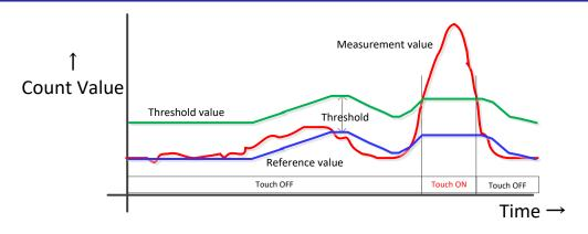
Figure 2 Button Touch Determination
