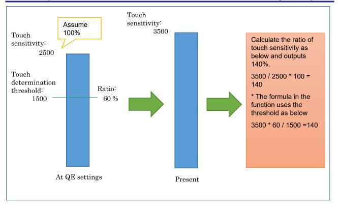
Following figure shows the case where an overlay panel is thicker and the touch sensitivity decreases.
