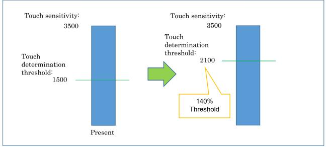
\*p\_touch\_sensitivity\_ratio = 140 old\_threshold\_ratio = 60 new\_threshold\_ratio = 60 new\_hysteresis\_ratio = 5
