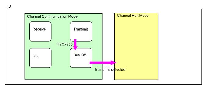
Figure 8-2 The operation when transitioning to channel halt mode at bus off entry (BOM[1:0] bit is B' 01)
