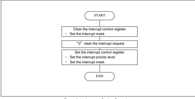
Figure 9-1 Interrupt Setting Procedure
