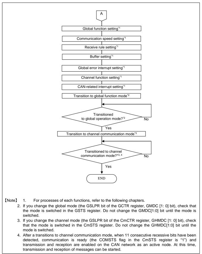
Figure 1-2 Procedure of CAN Configuration after resetting MCU 2/2
