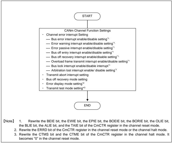
Figure 8-6 Channel Function Setting Procedure
