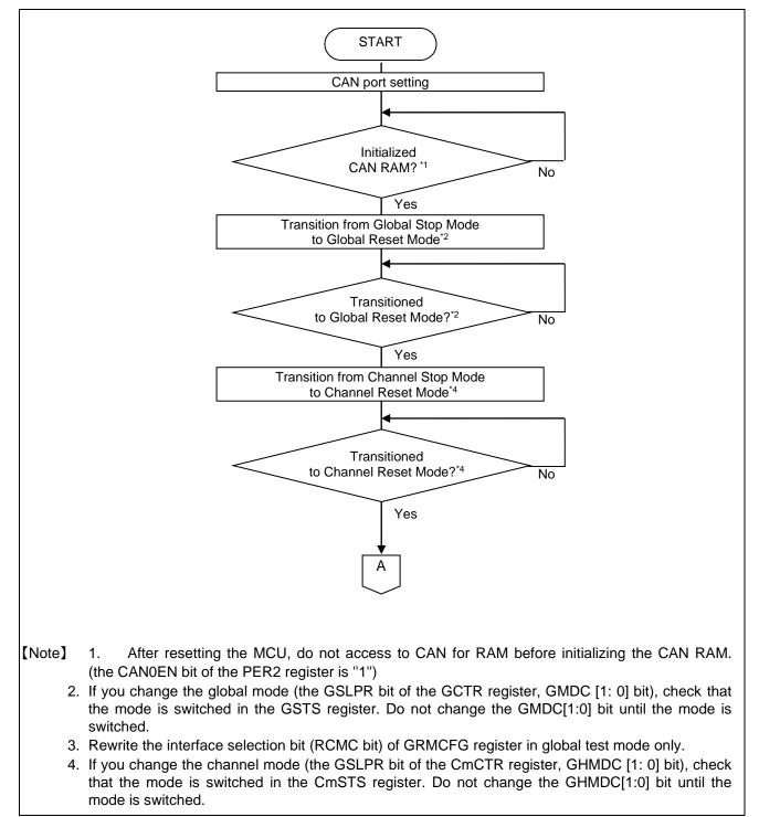
Figure 1-1 Procedure of CAN Configuration after resetting MCU 1/2
