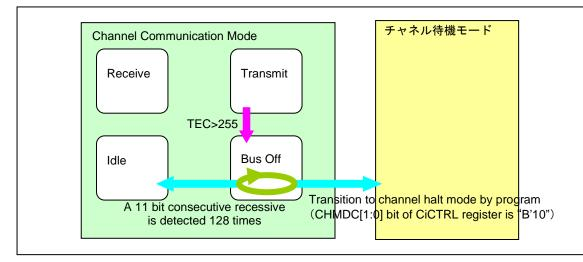
Figure 8-4 The operation when transitioning to channel halt mode by program request at bas off (BOM[1:0] bit is B' 11)
