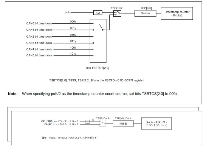
Figure 4-1 Timestamp Function Block Diagram
