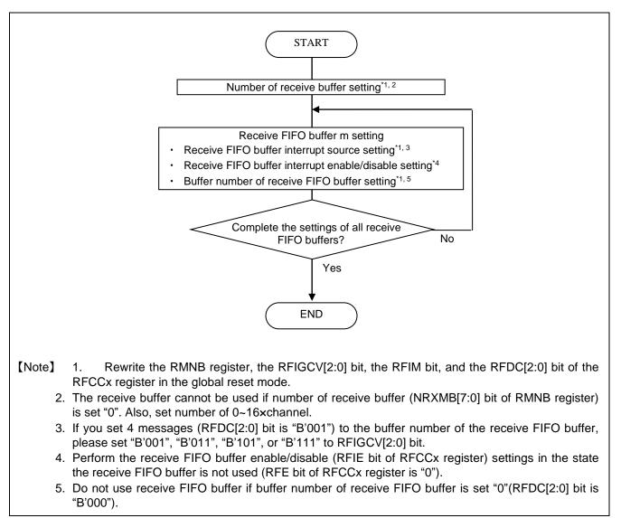
Figure 6-2 Receive Buffer and Receive FIFO Buffer Setting Procedures
