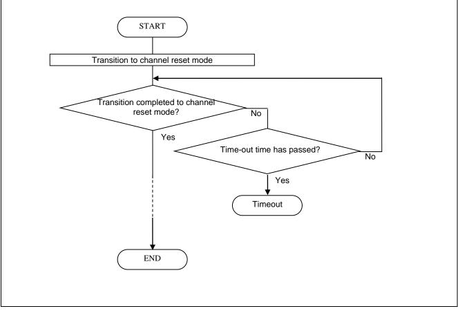
Figure 11-1 Example of Processing with Loop Time Limit
