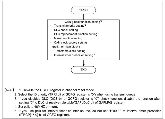
Figure 4-2 Global Function Setting Procedure
