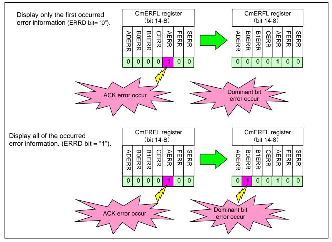
Figure 8-5 Operation Example of Error Display Mode
