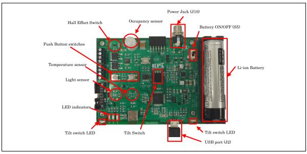
Figure 1 Sensor Panel board
