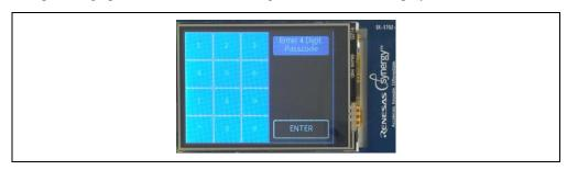
**Step 5.** The Login Screen has numeric key pad for entering password. Type 1234 using keypad and press ENTER button.
