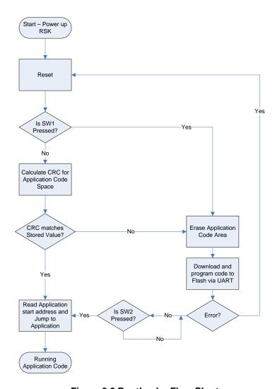
Figure 3.2 Bootloader Flow Chart
