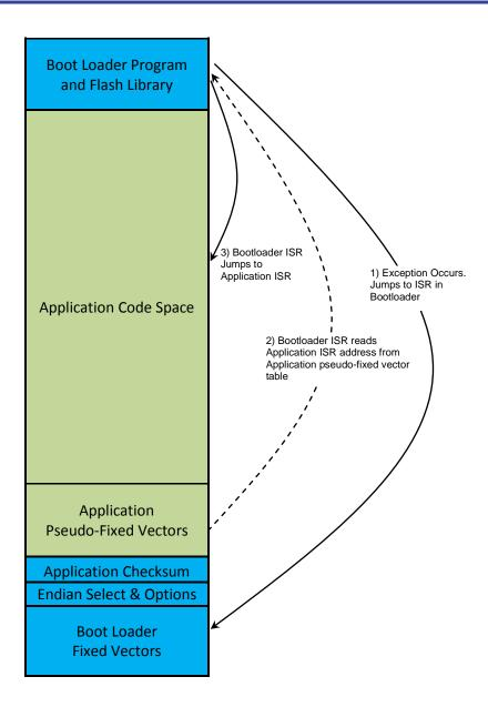
**Figure 4.1 Application Interrupt Forwarding Process**
