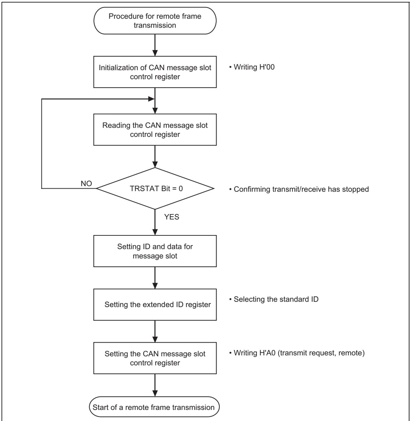
Figure 4.3.1 Remote Frame Transmission Processing
