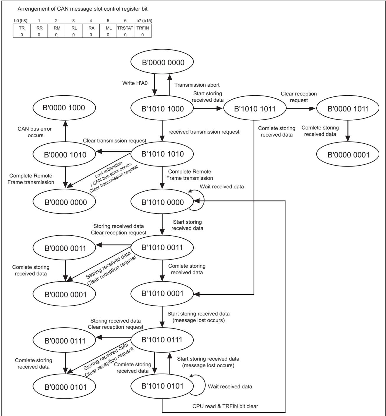
Figure 4.4.1 The State of CAN Message Slot Control Registers during Remote Frame Transmission
