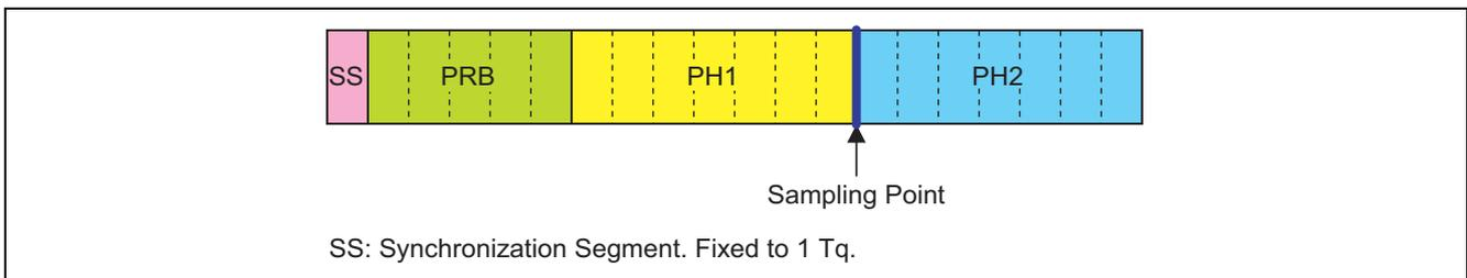
Figure 4.5.1 Bit Timing
