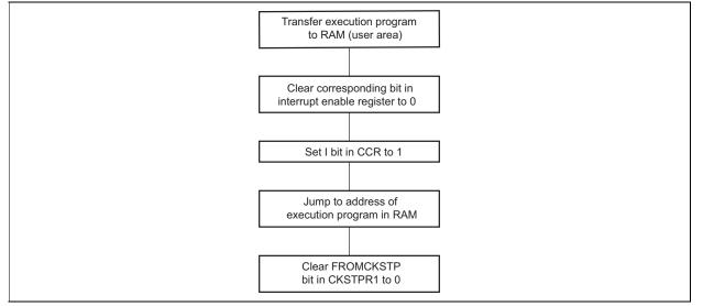
Figure 3 Configuring Module Standby Mode (Without Using the RAM Emulation)
