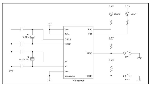
Figure 1 Hardware Block Diagram (Renesas Starter Kit for H8/38099)
