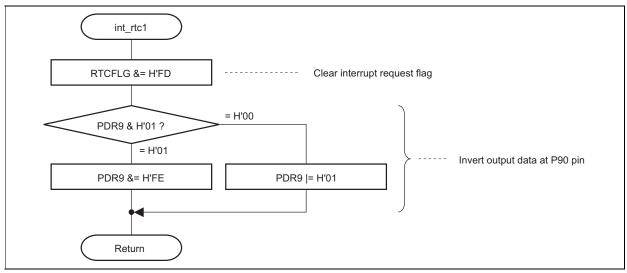
Figure 9 int\_rtc1 Function (RTC 0.5 s Overflow Interrupt Processing Routine) Flowchart
