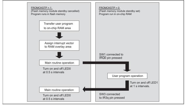
Figure 4 State Transition Diagram
