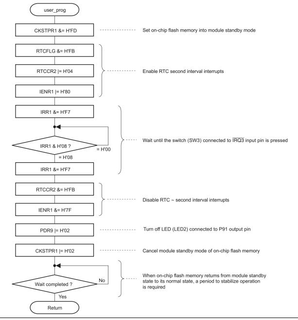
Figure 11 user\_prog Function (User Program Subroutine) Flowchart
