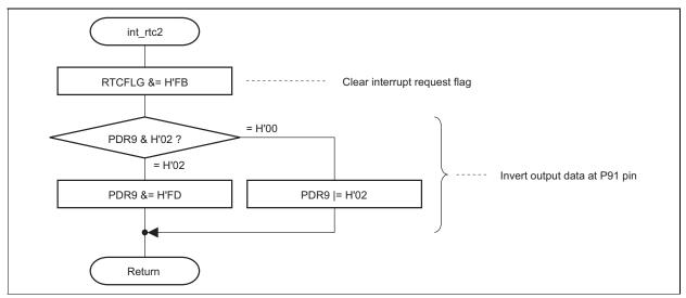
Figure 10 int\_rtc2 Function (RTC Second Interval Interrupt Processing Routine) Flowchart
