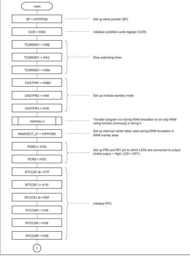
Figure 8 main Function (Main Routine) Flowchart
