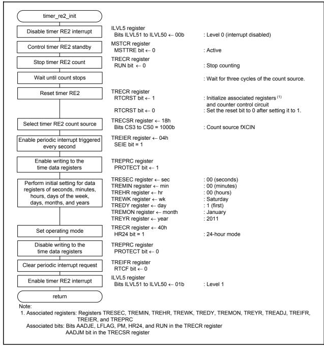
Figure 3.4 Initial Setting of Timer RE2
