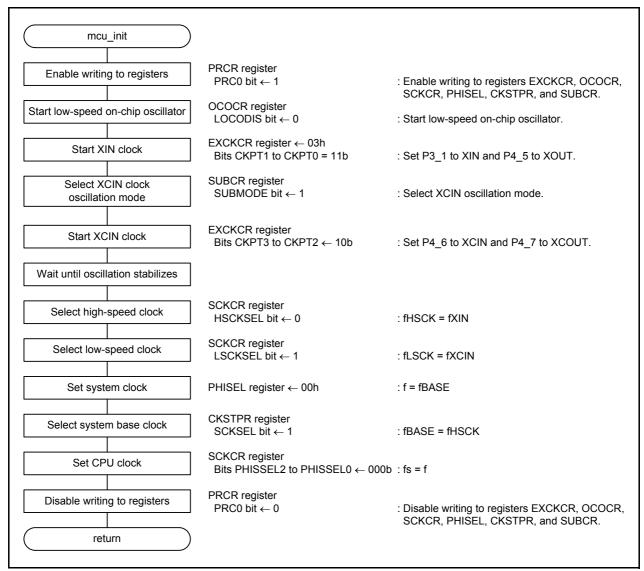
Figure 3.3 System Clock Setting
