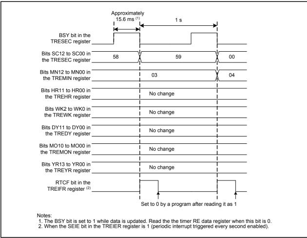
Figure 3.1 Real-Time Clock Operation
