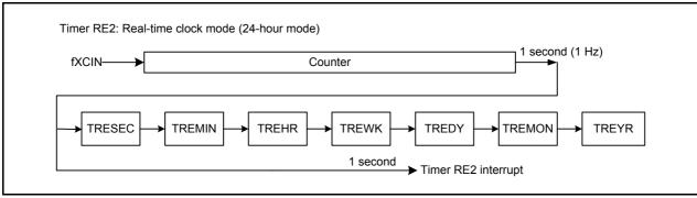
Figure 1.1 Block Diagram
