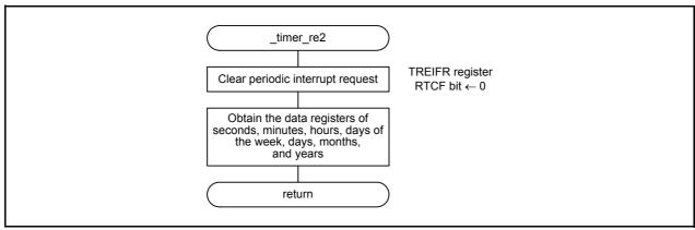
Figure 3.5 Timer RE2 Interrupt Handling
