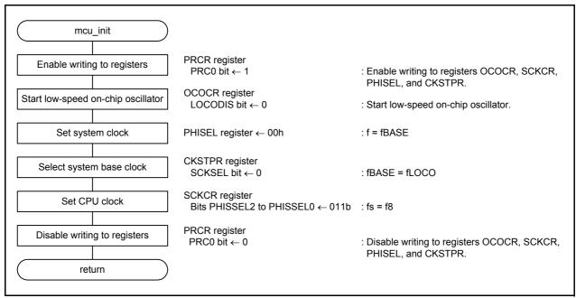
Figure 5.3 System Clock Setting
