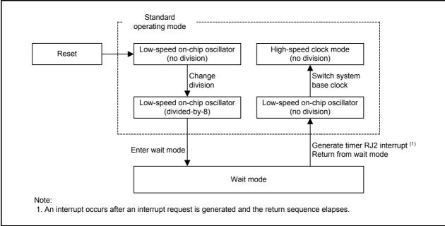
Figure 1.2 Usage Example for Sample Program 2
