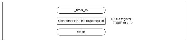
Figure 4.10 Timer RB2 Interrupt Handling
