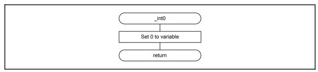
Figure 4.9 INTO Interrupt Handling
