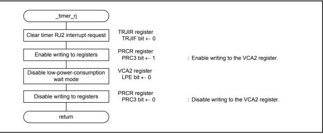
Figure 5.7 Timer RJ2 Interrupt Handling
