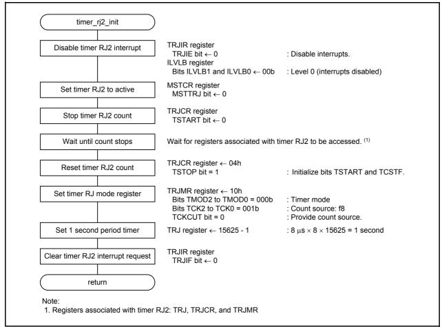
Figure 5.4 Initial Setting of Timer RJ2
