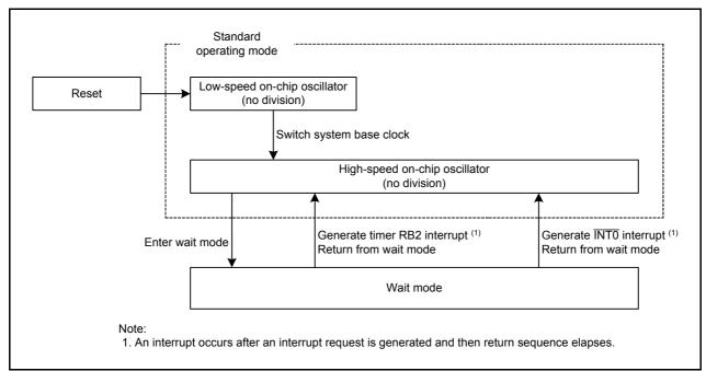
Figure 1.1 Usage Example for Sample Program 1
