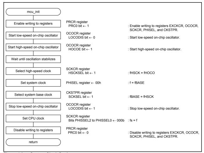
Figure 4.3 System Clock Setting
