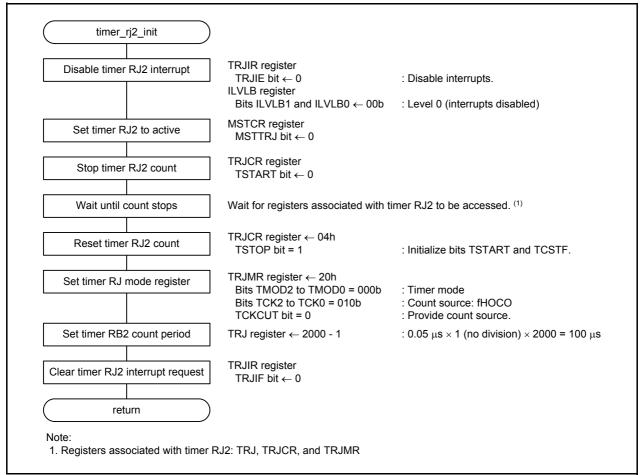
Figure 4.5 Initial Setting of Timer RJ2
