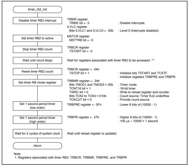
Figure 4.6 Initial Setting of Timer RB2
