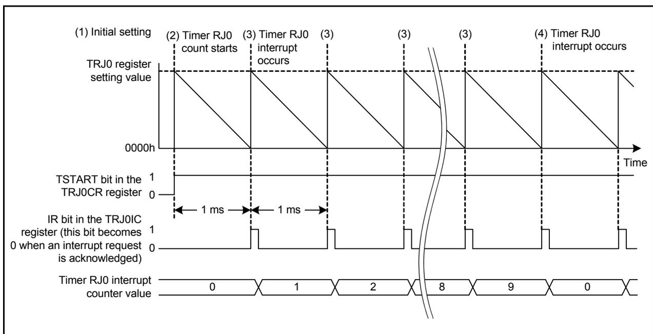
Figure 3.1 Timing Diagram
