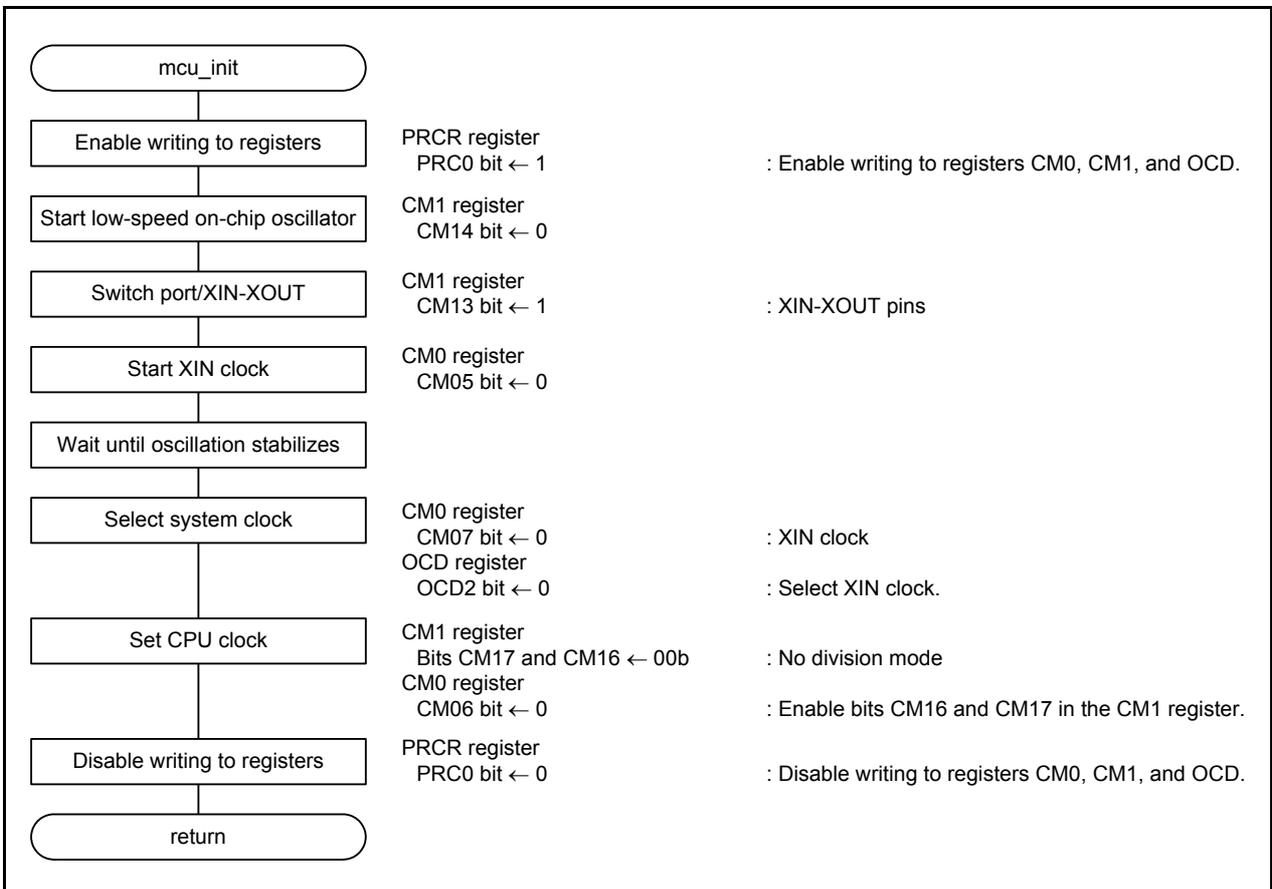
Figure 3.3 System Clock Setting
