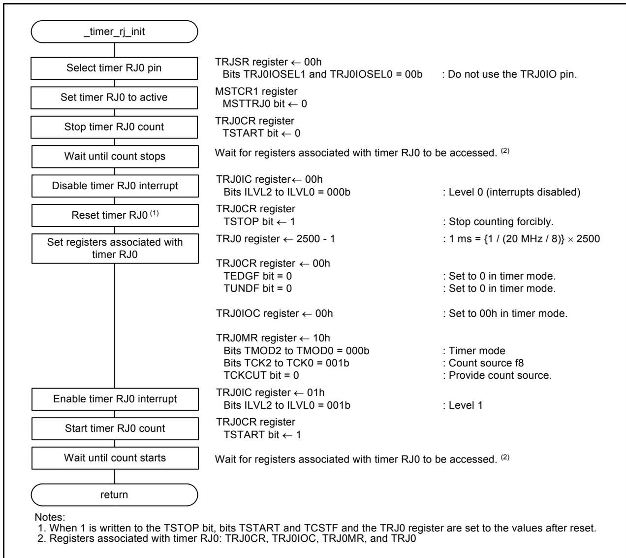
Figure 3.4 Initial Setting of Timer RJ0
