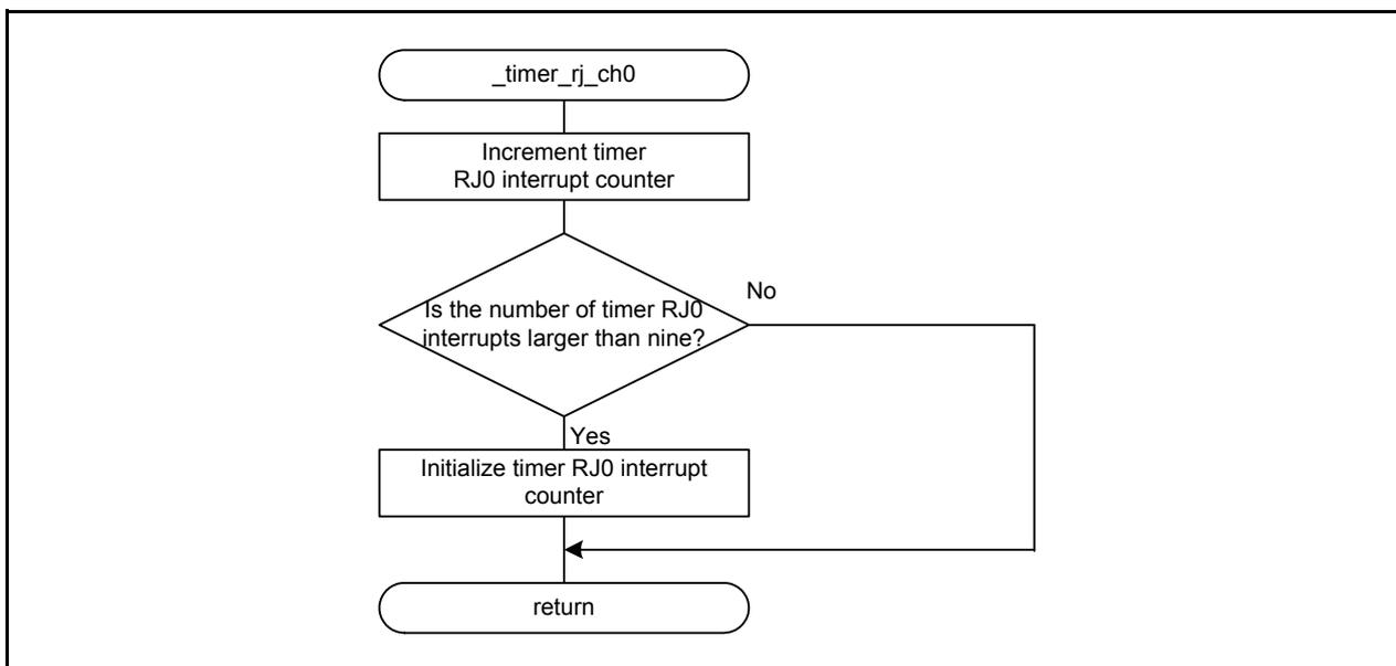
Figure 3.5 Timer RJ0 Interrupt Handling
