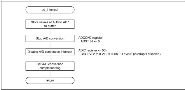
Figure 4.11 A/D Interrupt Handling
