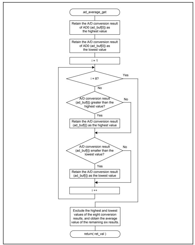
Figure 4.9 Obtaining the Average A/D Value
