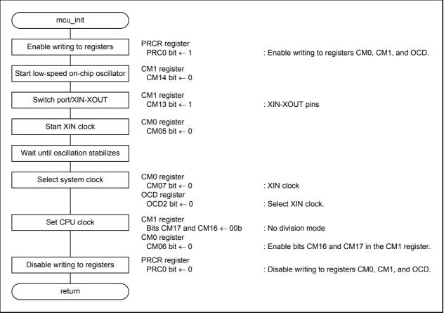
Figure 4.4 System Clock Setting
