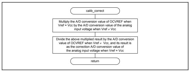
Figure 4.10 Calculating the Correction Value
