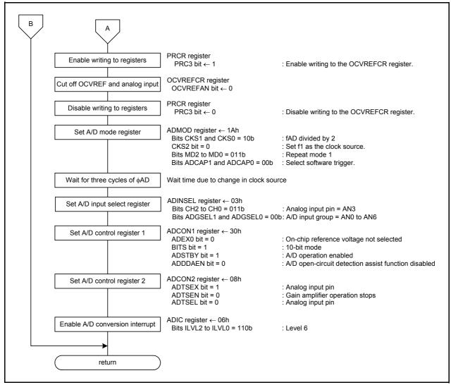
Figure 4.6 Initial Setting of the A/D Converter (2/2)
