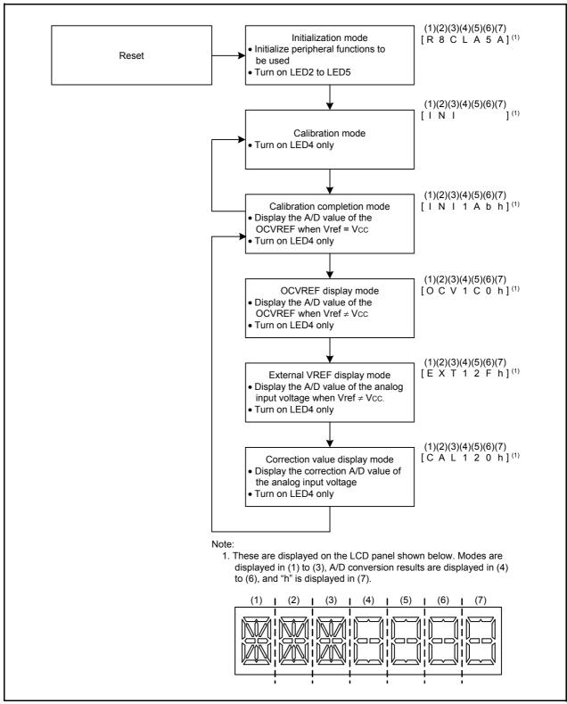
Figure 1.2 Mode Block Diagram
