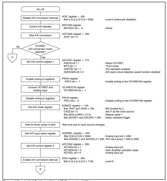
Figure 4.5 Initial Setting of the A/D Converter (1/2)
