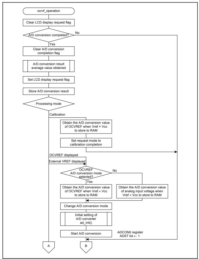
Figure 4.7 On-Chip Reference Voltage Processing (1/2)
