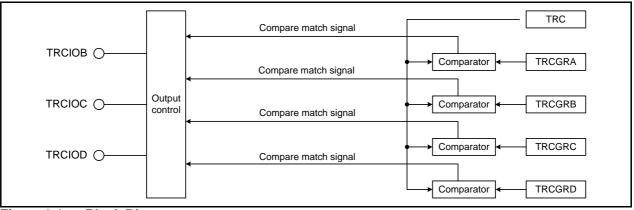
Figure 3.1 Block Diagram
