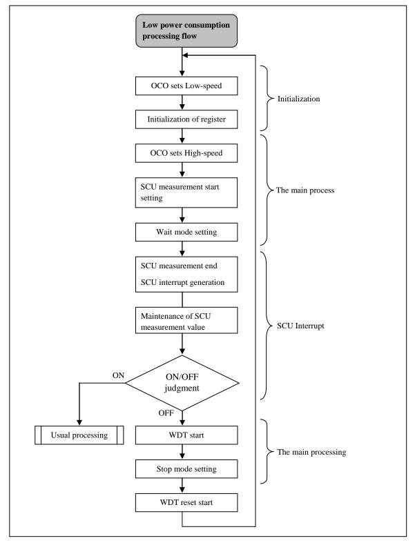
Figure 9 Processing flow for low power consumption (Watchdog timer use)
