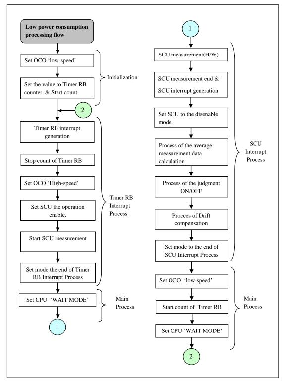
Figure 1 Processing flow for low power consumption
