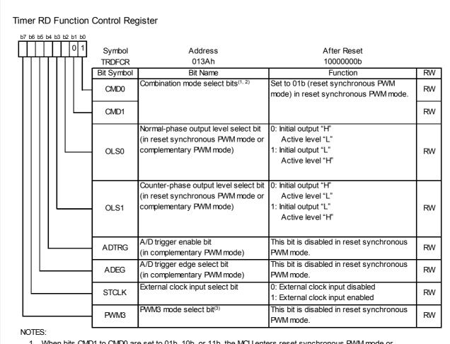
1. When bits CMD1 to CMD0 are set to 01b, 10b, or 11b, the MCU enters reset synchronous PWM mode or complementary PWM mode regardless of the setting of the TRDPMR register.
