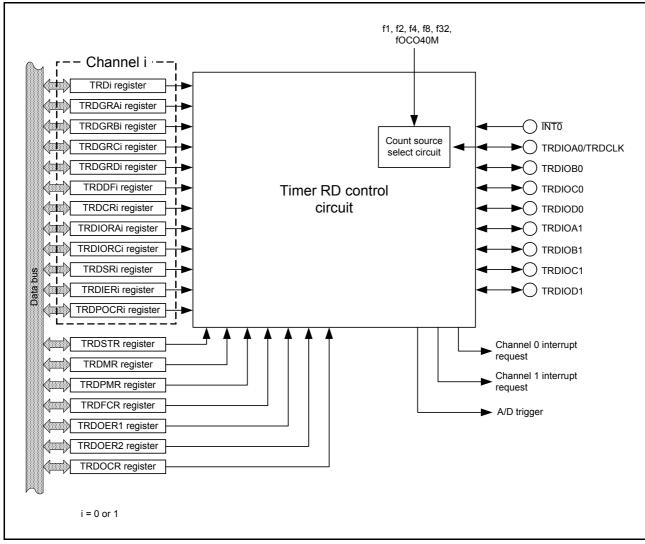
Figure 3.1 Block Diagram of Timer RD
