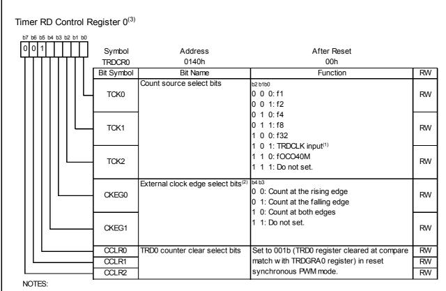
1. This setting is enabled when the STCLK bit in the TRDFCR register is set to 1 (external clock input enabled).
