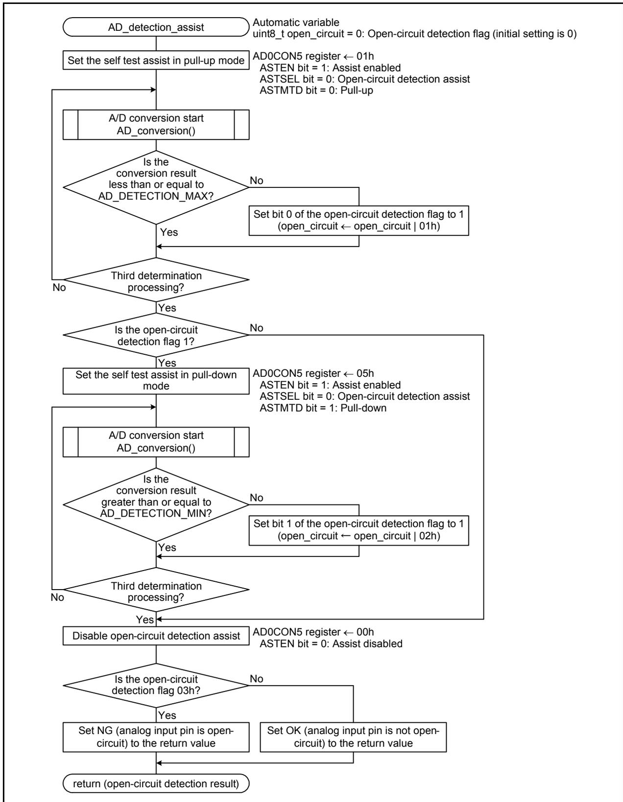
Figure 5.6 Detecting Open-Circuit in an Analog Input Pin
