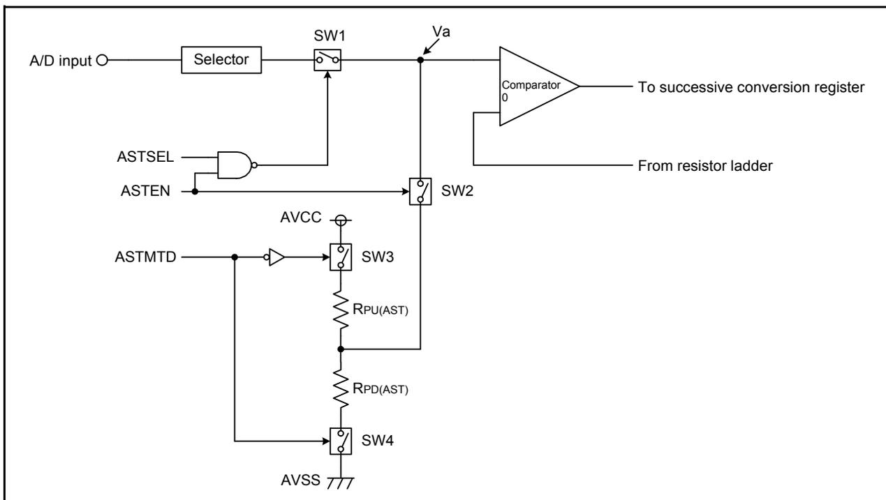
**Figure 5.1 Block Diagram of the Open-Circuit Detection Assist Circuit**
