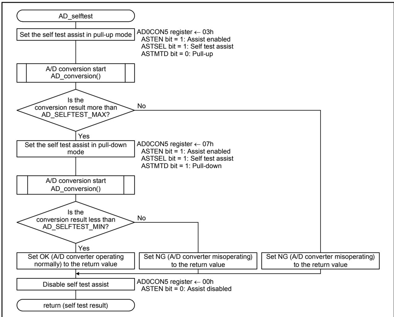
Figure 5.5 A/D Converter Self Test
