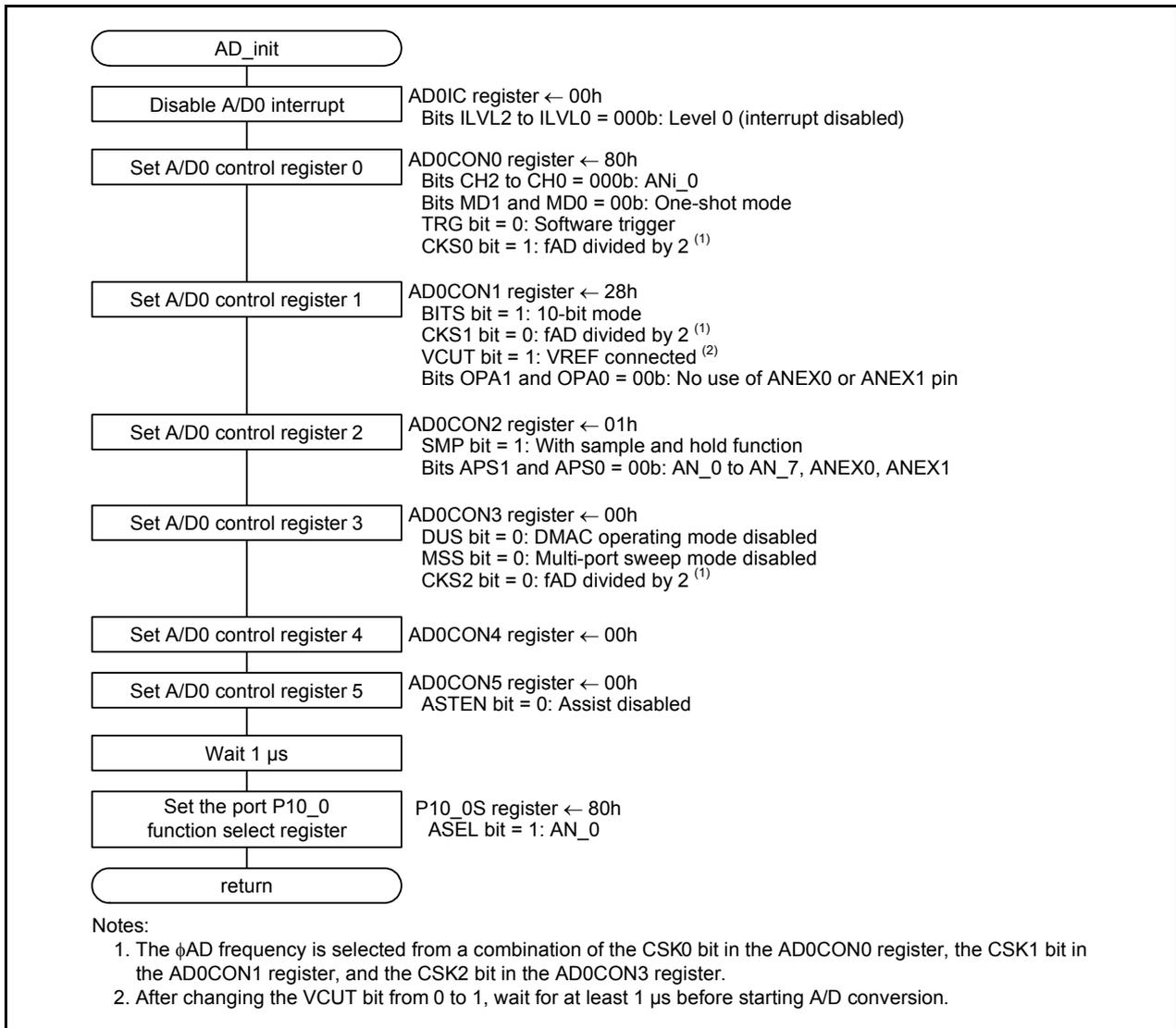
**Figure 5.3 A/D Converter Initialization**
