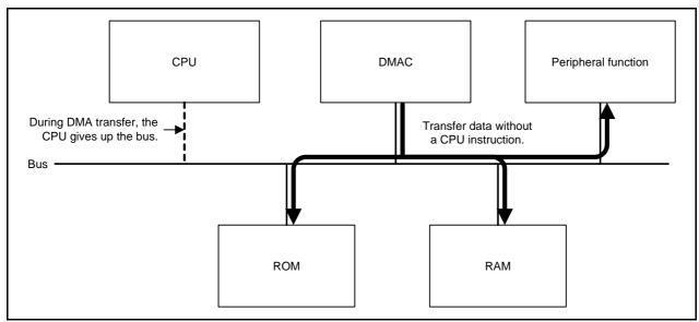
Figure 1.1 Block Diagram
