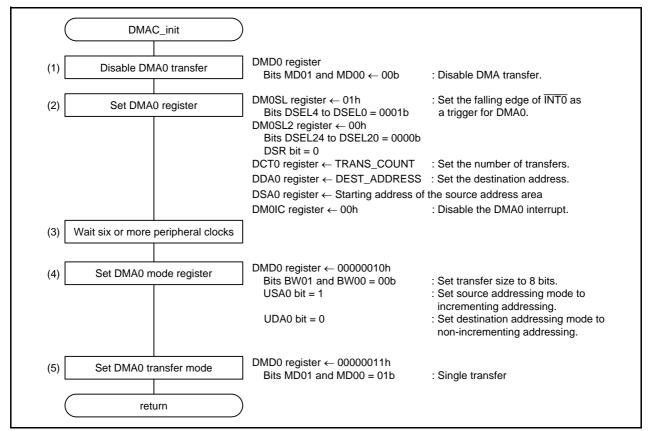
Figure 5.3 DMAC Initial Setting
