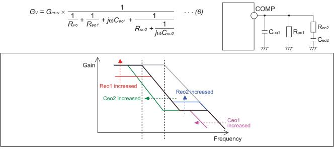
Figure 10 Overview of Gain–Frequency Characteristics
