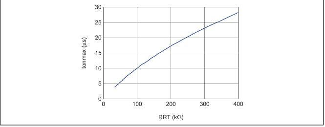
Figure 8 RRT-tonmax Characteristics
