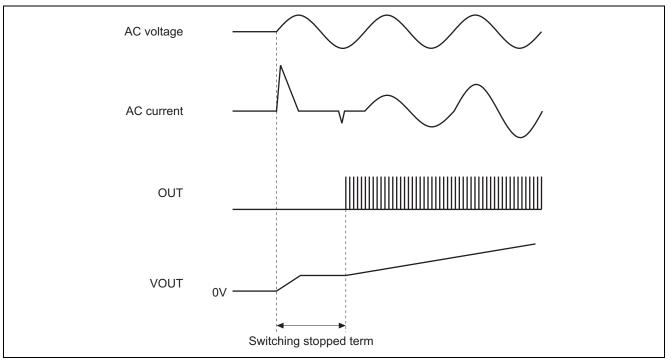
Figure 7 Example(1) Stop of the Switching Operation
