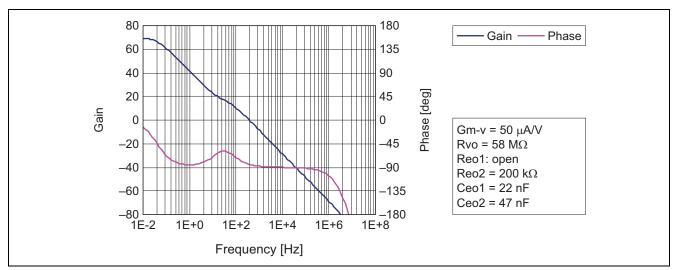
Figure 11 Frequency Characteristics of the Error Amplifier
