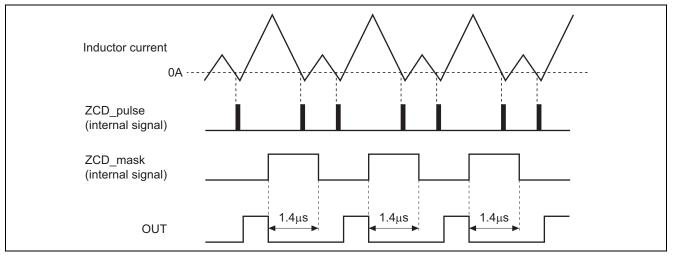
Figure 6 Example of Off Time Control
