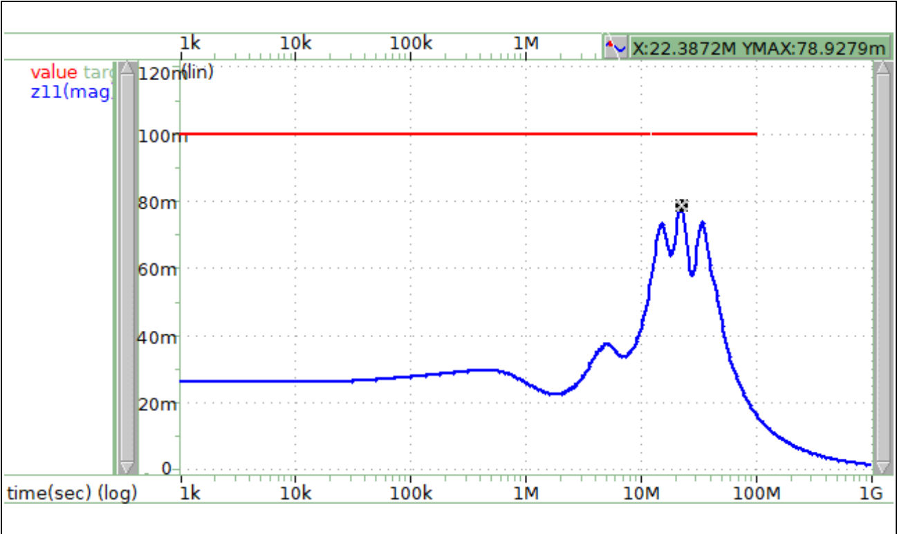
Figure 4.4 Target impedance of core power supply and impedance data of 21mm RZ/G2L
