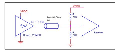
Figure 2 LVCMOS Parallel Termination
