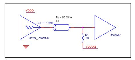
Figure 1 LVCMOS Driver Standard Termination
