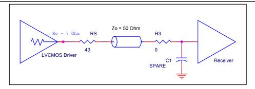
Figure 4 One to One LVCMOS Series Termination
