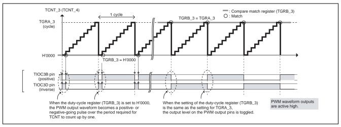
Figure 5 Settings of the Duty-Cycle Register and Corresponding PWM Output Waveforms
