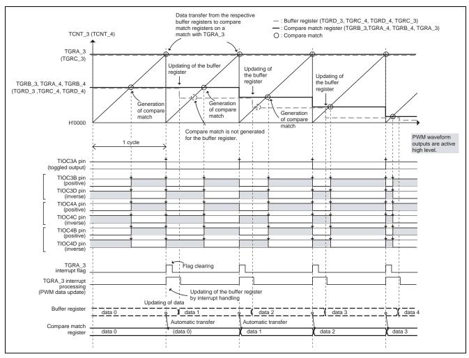
Figure 4 Operation (Buffered Operation) in Reset-Synchronized PWM Mode
