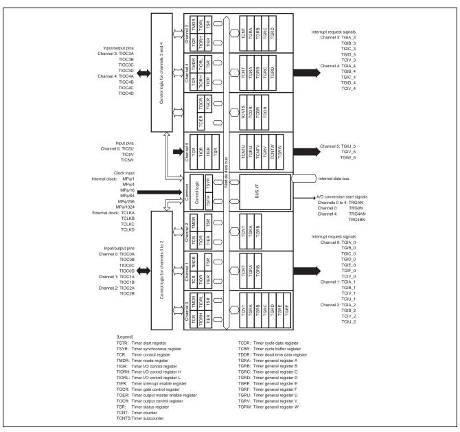
Figure 2 Block Diagram of MTU2
