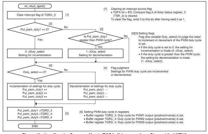
Figure 10 Handling the Compare Match (TGRA\_3) Interrupt from Channel 3 of MTU2
