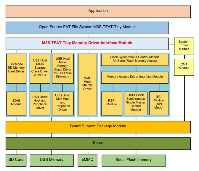
Fig.1-1 Structure of software
