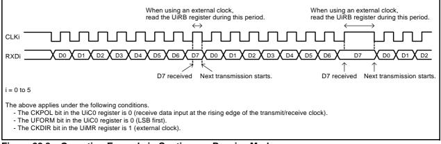
Figure 22.8 Operation Example in Continuous Receive Mode
