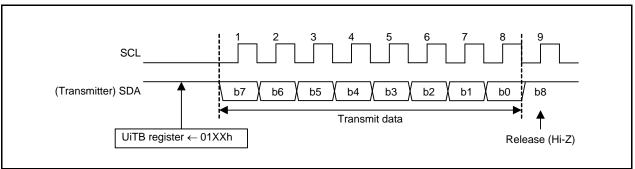
Figure 4.8 Byte Data Transmission
