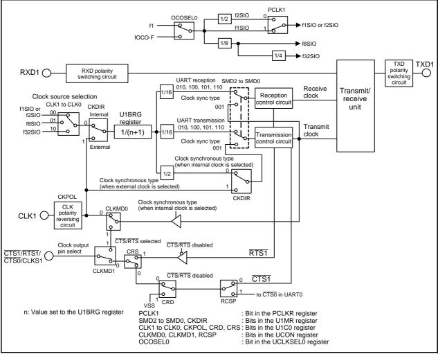
Figure 22.2 UART1 Block Diagram
