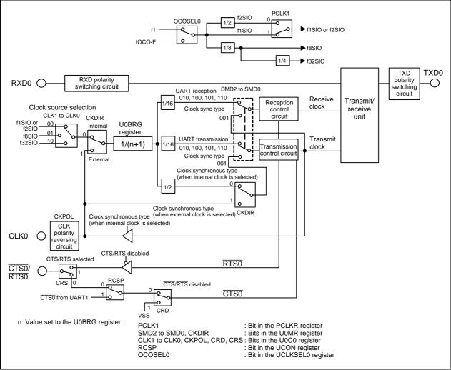
Figure 22.1 UART0 Block Diagram
