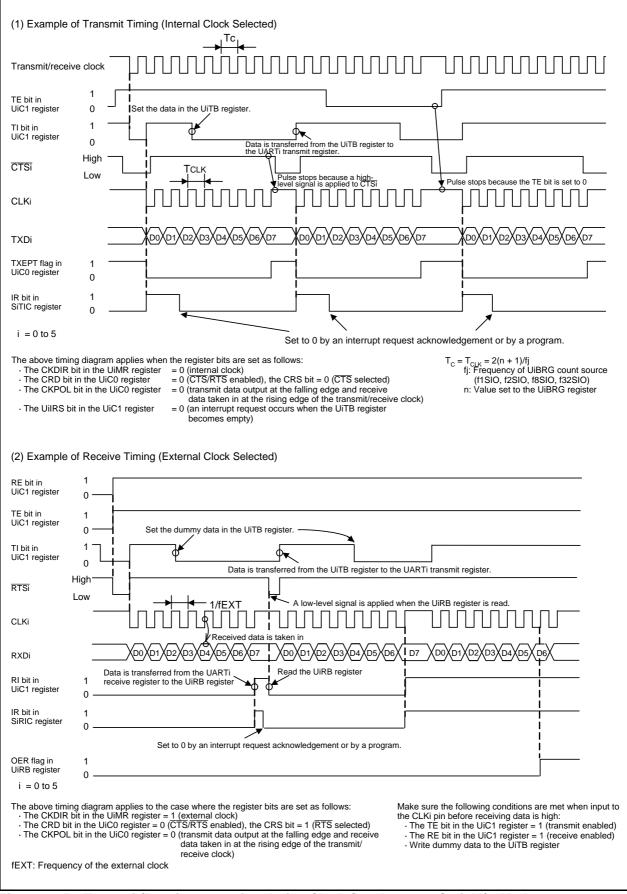
Figure 22.5 Transmit/Receive Operation during Clock Synchronous Serial I/O Mode
