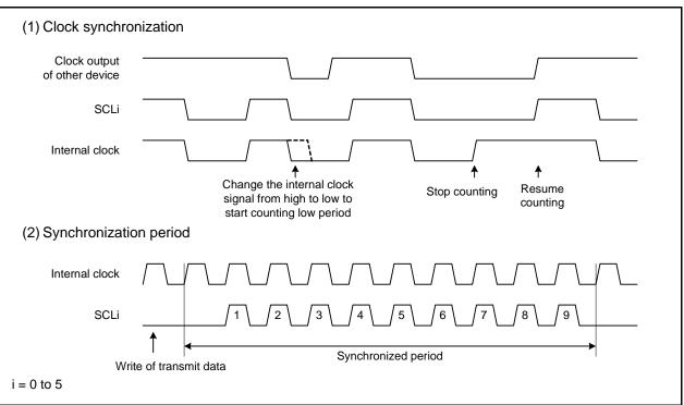
Figure 4.5 Clock Synchronization
