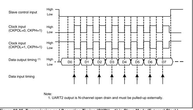
Figure 22.25 Transmission and Reception Timing (CKPH = 1) in Slave Mode (External Clock)
