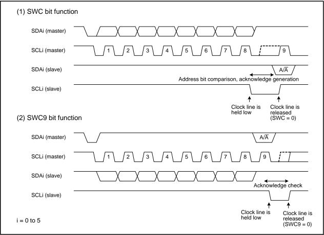
Figure 4.4 Inserting Wait-states Using Bits SWC and SWC9
