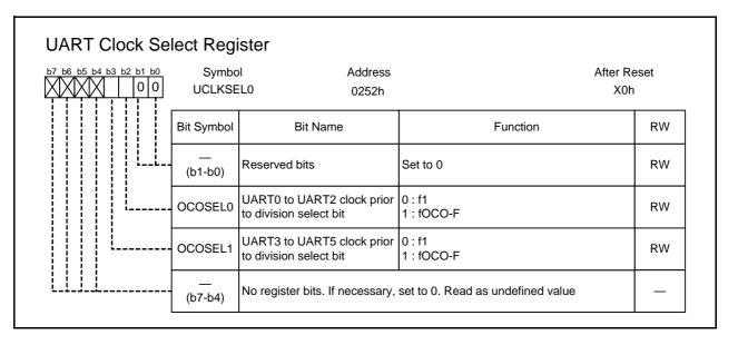
OCOSEL0 (UART0 to UART2 clock prior to division select bit) (b2) OCOSEL1 (UART3 to UART 5 clock prior to division select bit) (b3)
