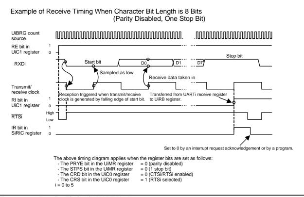
Figure 22.13 Receive Timing in UART Mode
