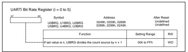
Write to the UiBRG register while serial interface is neither transmitting nor receiving. Use MOV instruction to write to the UiBRG register.
