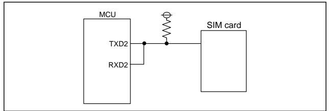
Figure 22.28 Example of SIM Interface Connection
