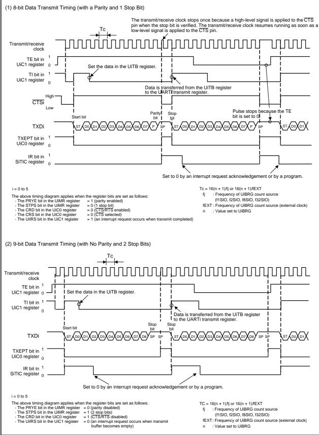
Figure 22.12 Transmit Timing in UART Mode
