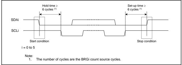
Figure 4.1 Detecting Start and Stop Conditions
