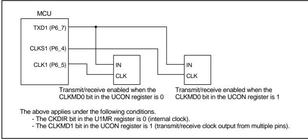
Figure 22.10 Transmit/Receive Clock Output from Multiple Pins
