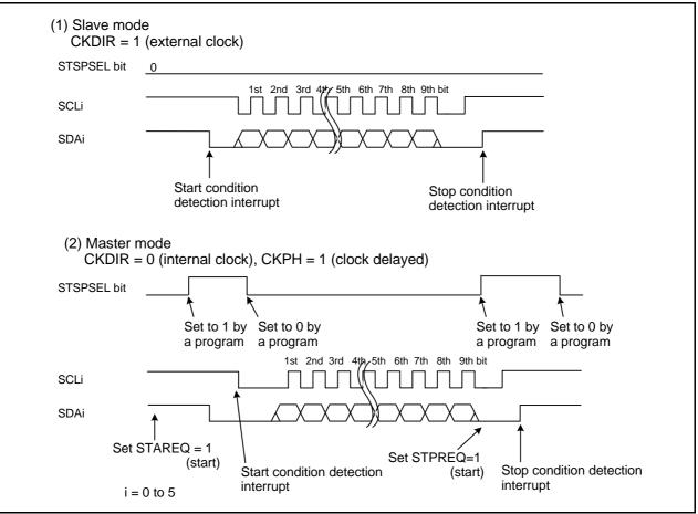
Figure 22.21 STSPSEL Bit Functions
