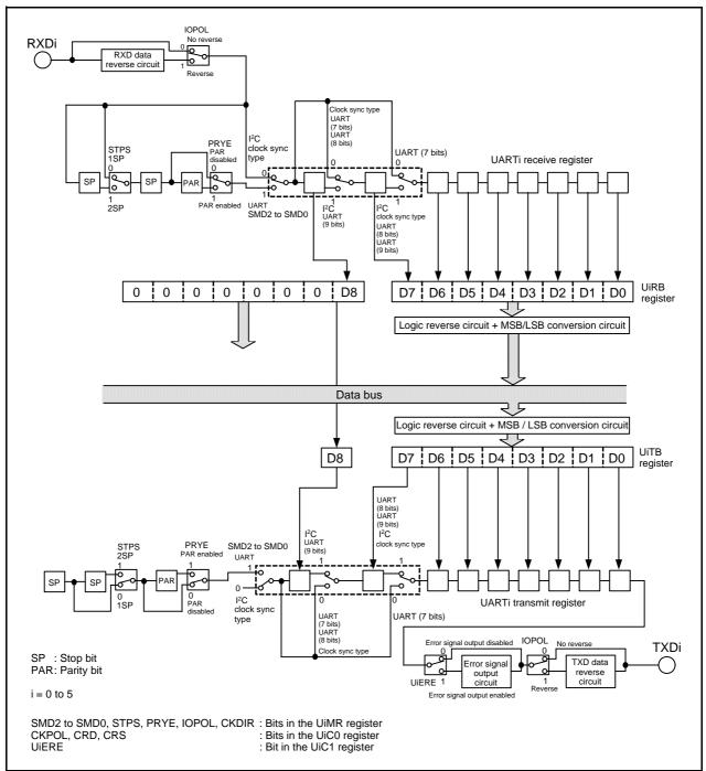
Figure 22.4 UARTi Transmit/Receive Unit Block Diagram
