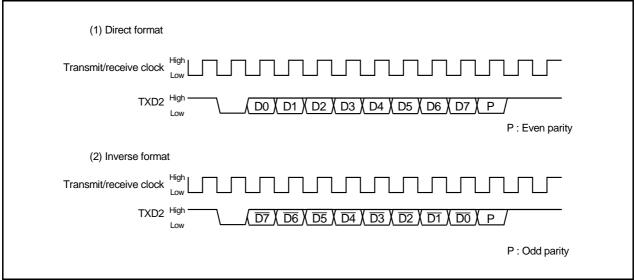
Figure 22.30 SIM Interface Format
