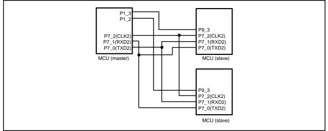
Figure 22.22 Serial Bus Communication Control Example (UART2)
