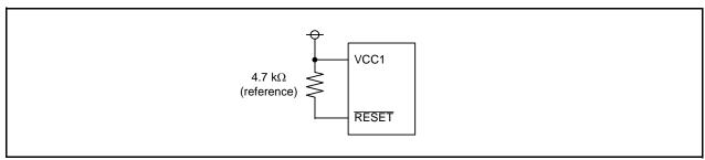
Figure 3.1 Power-On Reset Circuit
