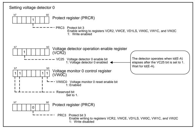
Figure 5.2 Setting Registers Associated with Voltage Monitor 0
