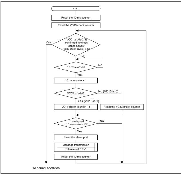
Figure 3.3 Determining When VCC1 ≥ Vdet2
