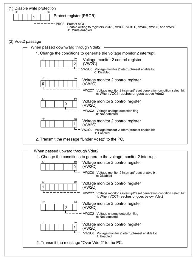
Figure 5.6 Interrupt Handling and Register Setting (1/2)
