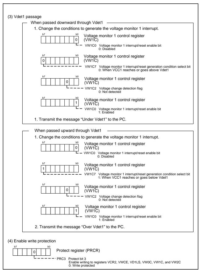
Figure 5.7 Interrupt Handling and Register Setting (2/2)
