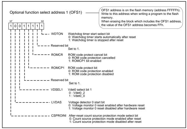
Figure 5.1 Setting Optional Function Select Address 1 (OFS1)
