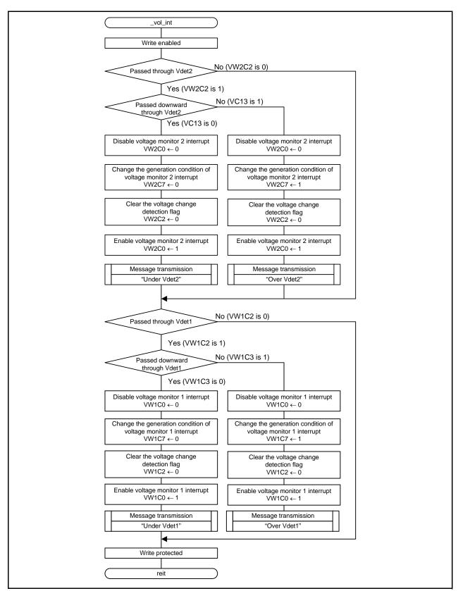
Figure 3.4 Determining the Voltage Monitor Interrupt Source
