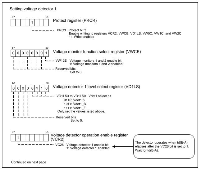
Figure 5.3 Setting Registers Associated with Voltage Monitor 1 (1/2)
