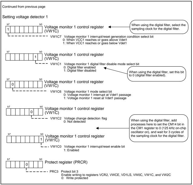
Figure 5.4 Setting Registers Associated with Voltage Monitor 1 (2/2)
