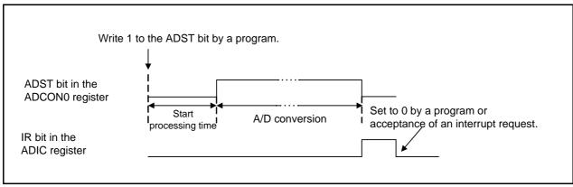
Figure 4.1 ADST Bit Operation
