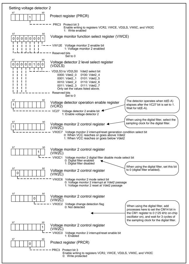
Figure 5.3 Setting Registers Associated with Voltage Monitor 2
