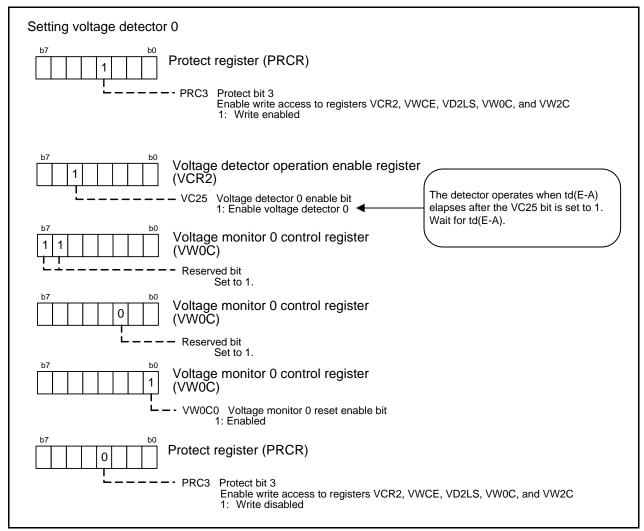
Figure 5.2 Setting Registers Associated with Voltage Monitor 0
