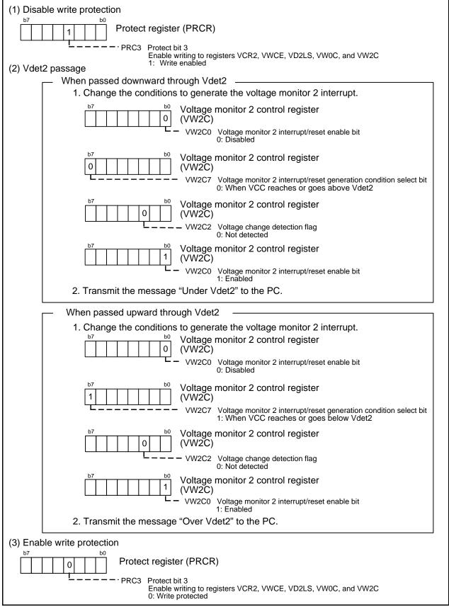
Figure 5.4 Interrupt Handling and Register Setting
