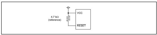
Figure 3.1 Power-On Reset Circuit
