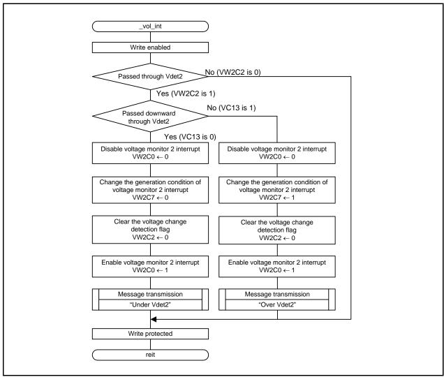
Figure 3.4 Determining the Voltage Monitor Interrupt Source
