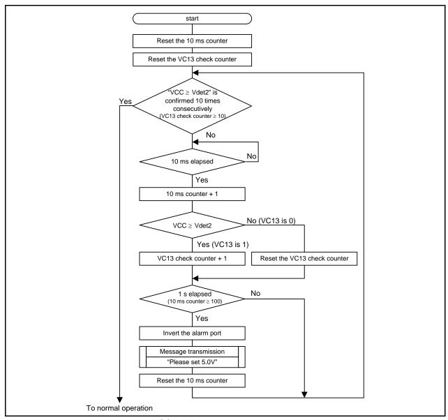
Figure 3.3 Determining When VCC ≥ Vdet2
