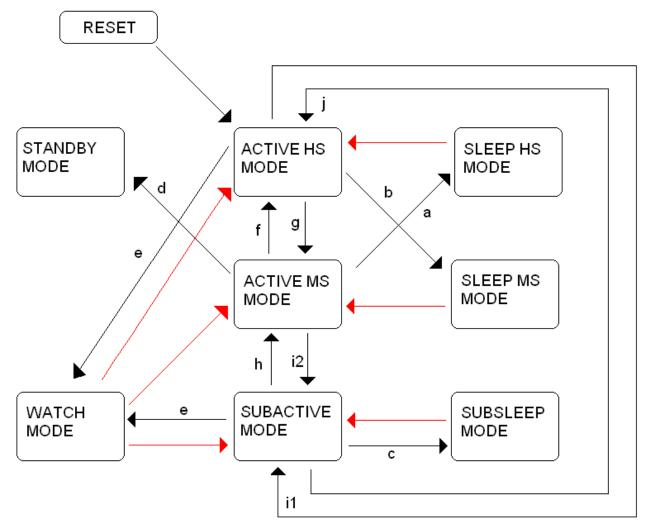
Figure 3: Power mode transitions used in the code
