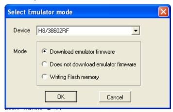
To download the ".mot" file using the Release configuration, click on the "connect" icon and select the third option in the window that appears.
