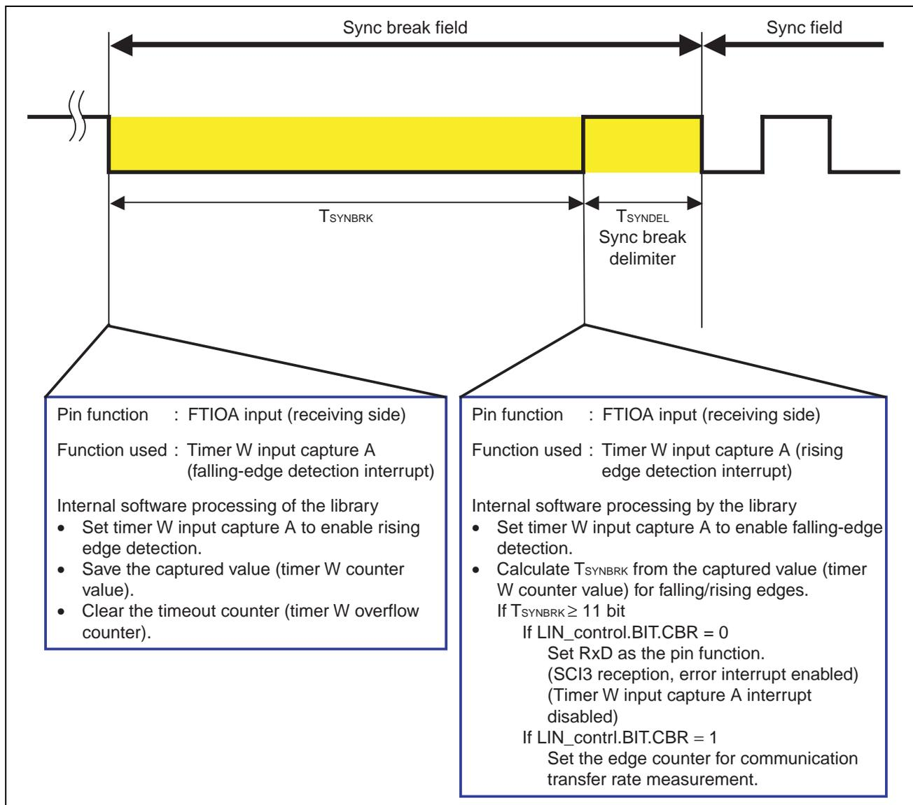
Figure 7 Detection of a Sync Break Field
