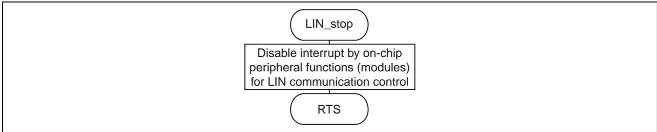
**Figure 16 Flowchart of the LIN Communication Control Stop Function**
