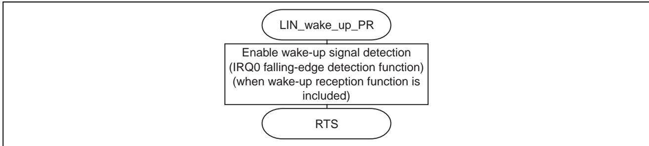
**Figure 19 Flowchart of the Wake-up Signal Reception Preparation Function**
