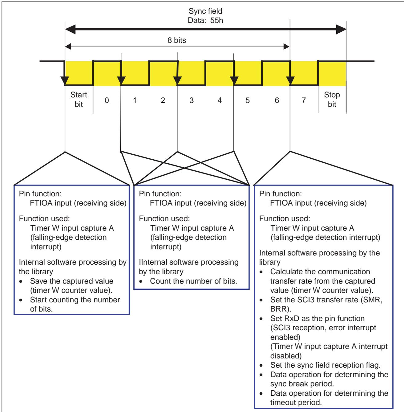
Figure 9 Correction of the Communication Transfer Rate by the Timer W Input Capture Function
