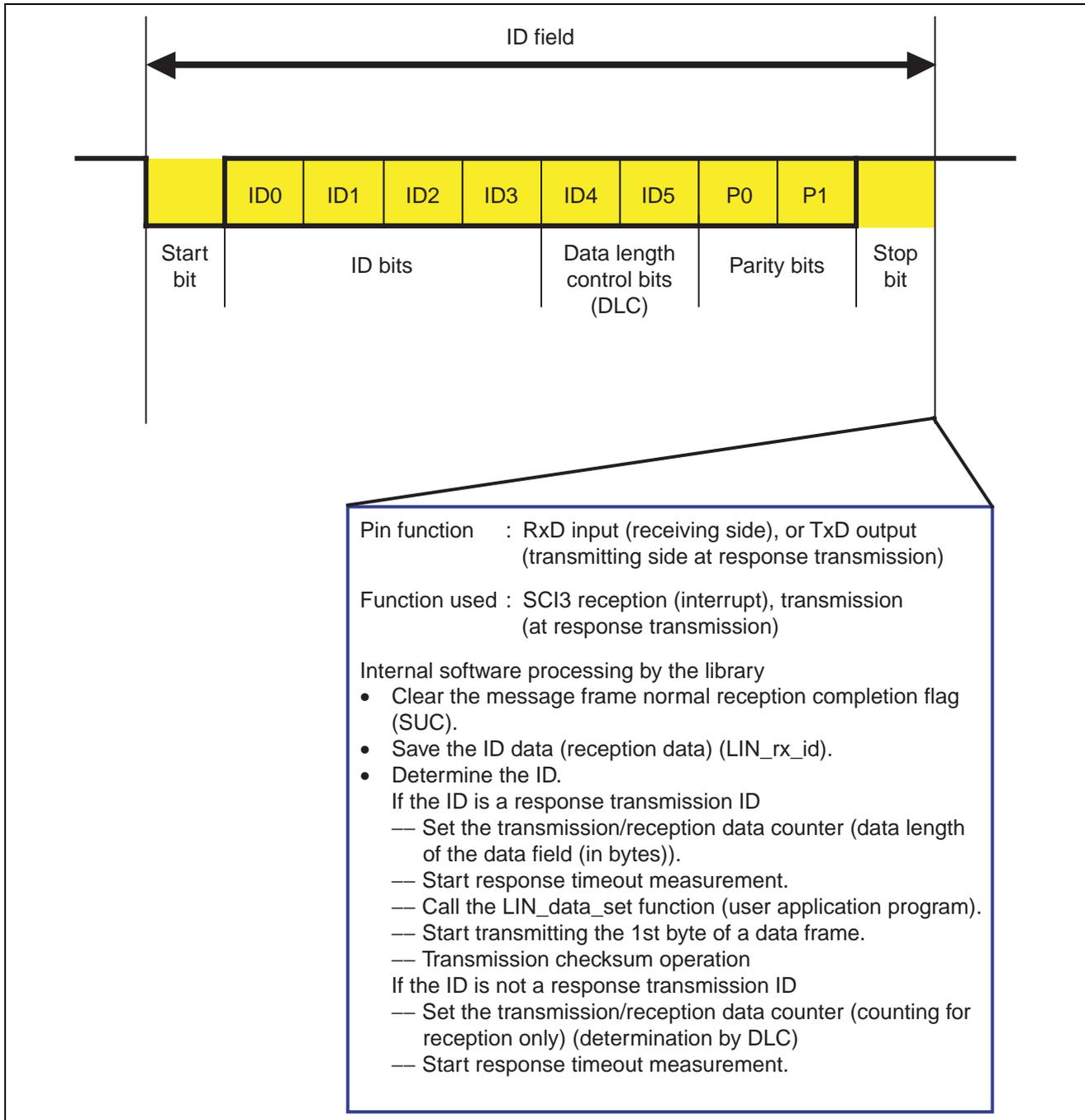
**Figure 10 ID Field Reception and Determination**
