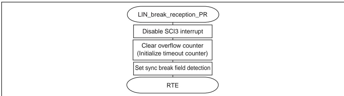
**Figure 20 Function for Preparing for Sync Break Field Detection and Reception**
