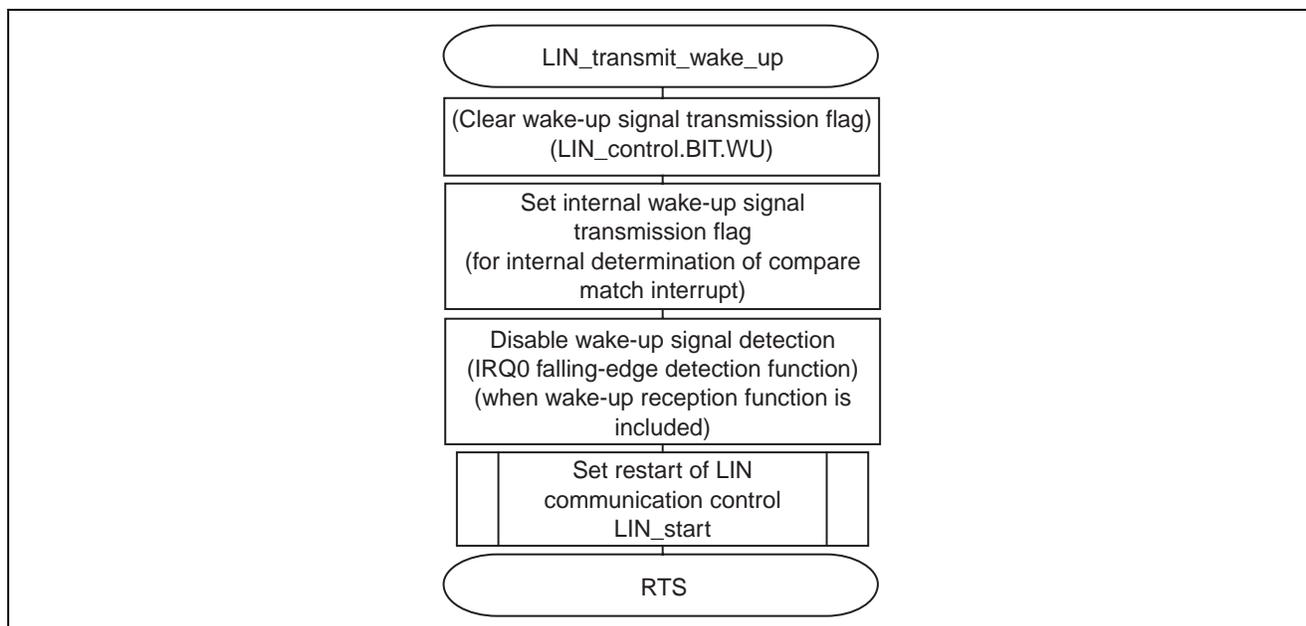
**Figure 18 Flowchart of the Wake-up Signal Transmission Function**
