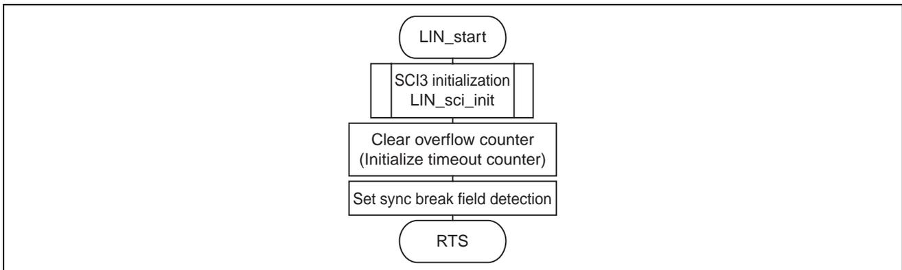
**Figure 17 Flowchart of the LIN Communication Control Restart Preparation Functions**
