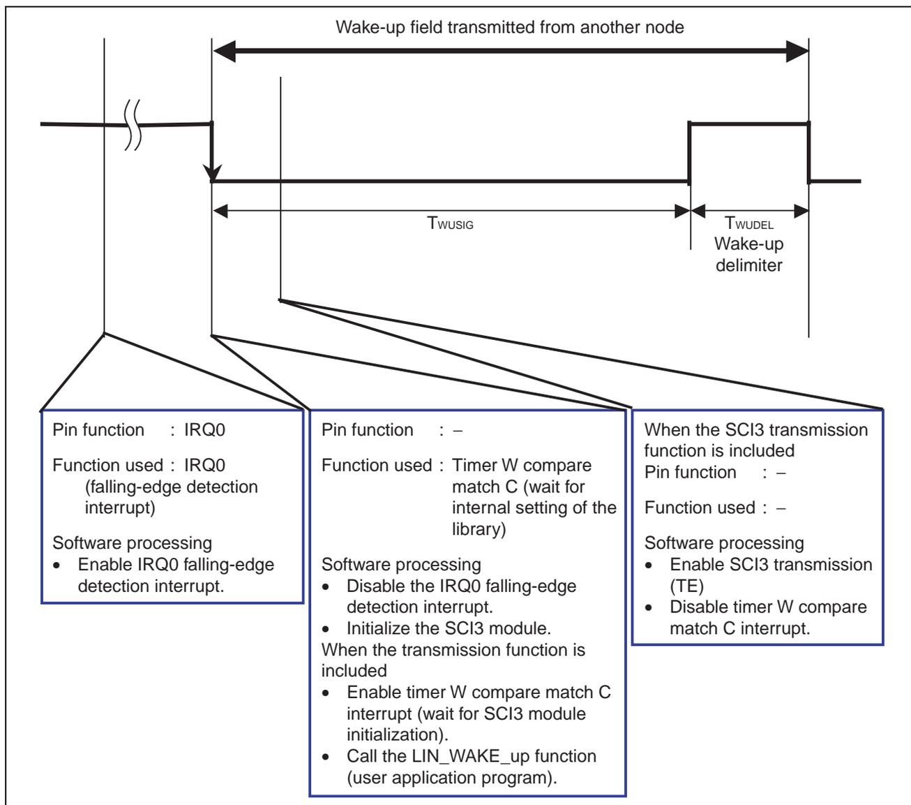
**Figure 14 Reception of a Wake-up Signal**
