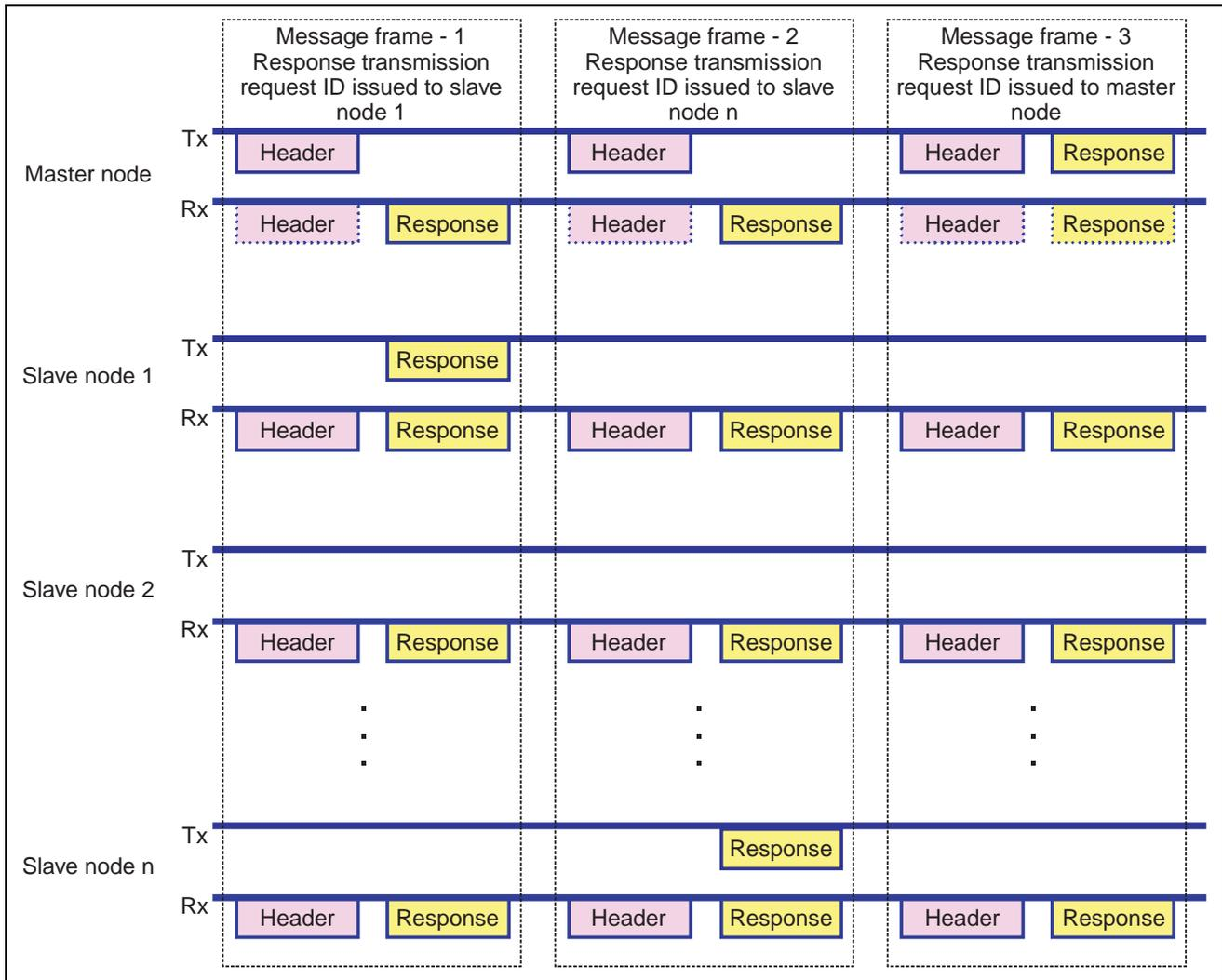
Figure 4 Transmission and Reception of Message Frames
