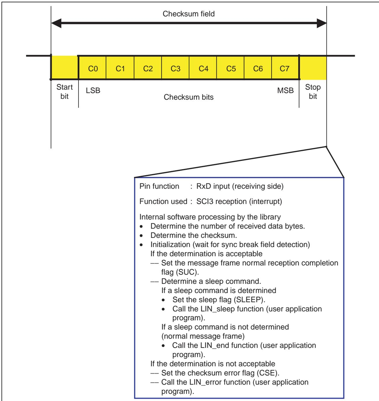
**Figure 12 Checksum Field Reception and Determination**
