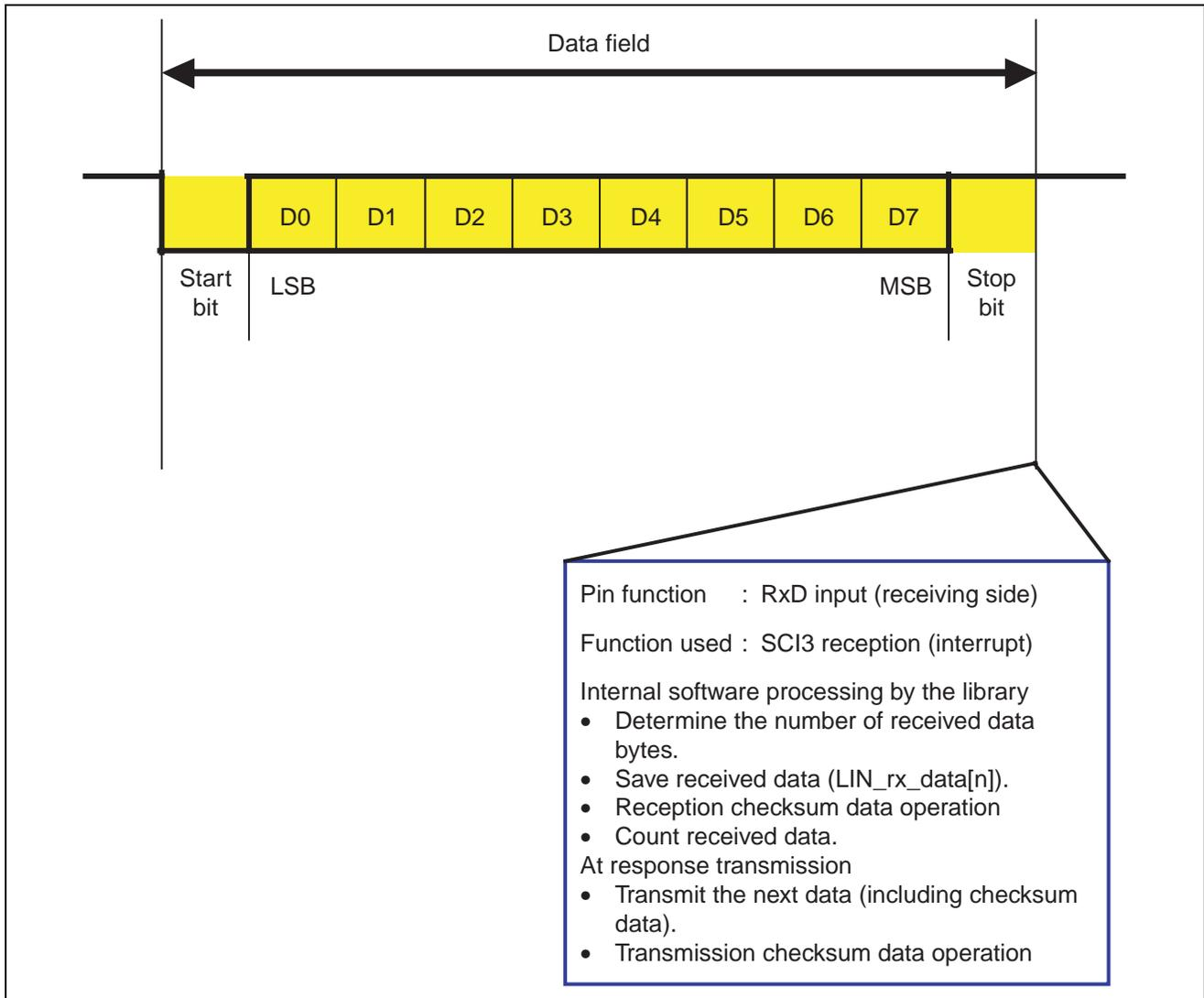
Figure 11 Transmission/Reception of a Data Field and Transmission of Checksum Data
