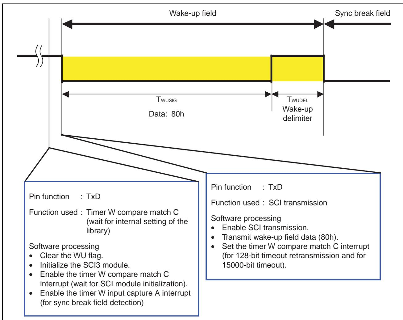
**Figure 13 Transmission of a Wake-up Signal**
