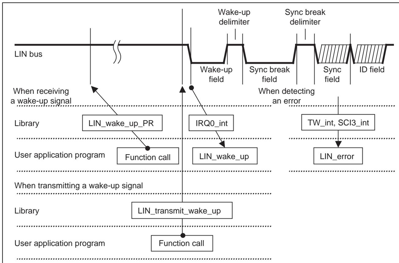
**Figure 6 Operation Overview at Error Detection and Wake-up Signal Transmission and Reception**
