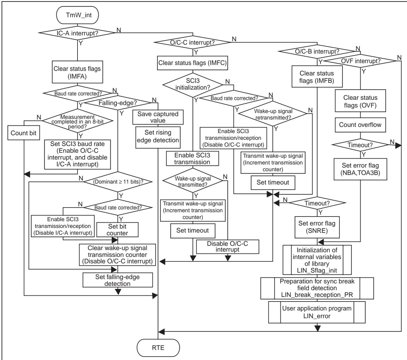
Figure 22 Flowchart of the Timer W Interrupt Function
