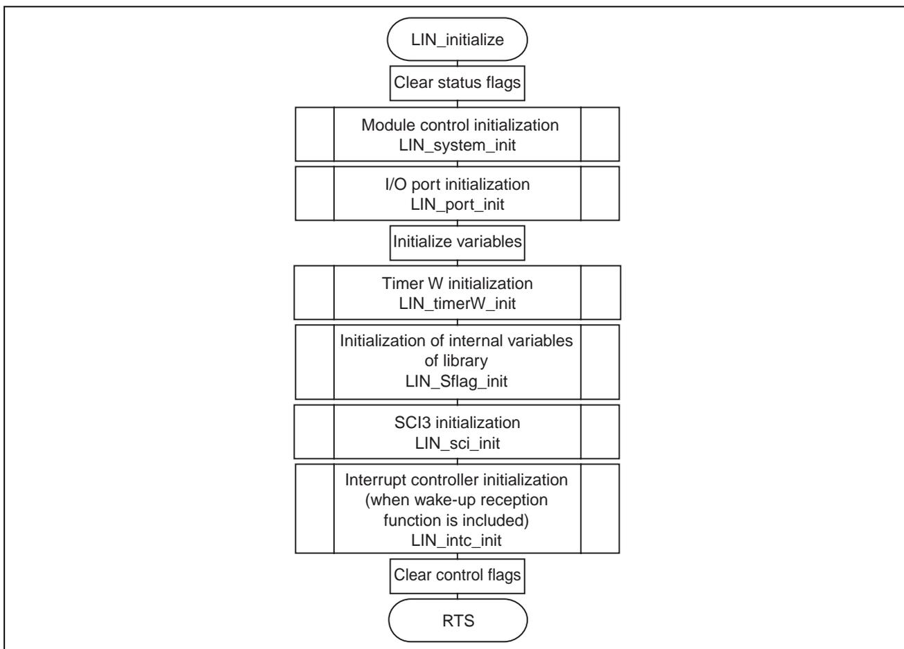
Figure 15 Initialization Function Flowchart
