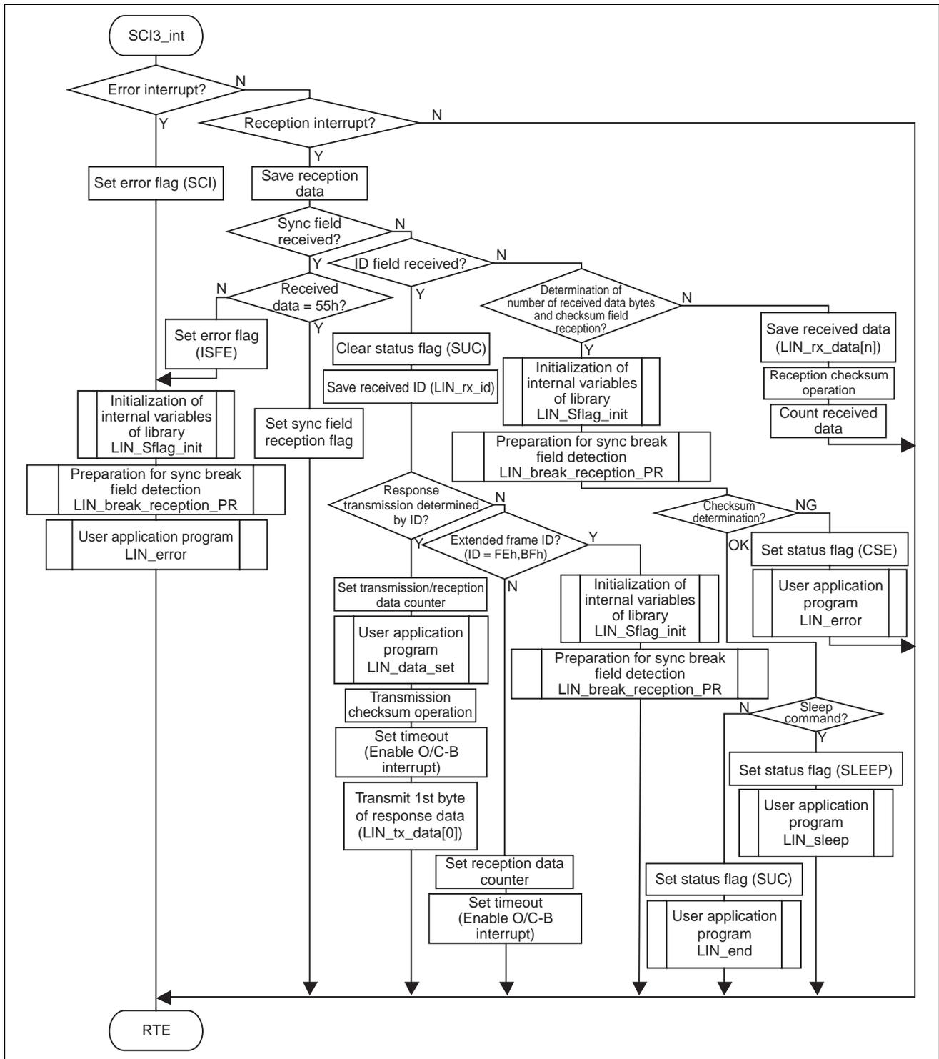
Figure 23 Flowchart of the SCI3 Interrupt Function
