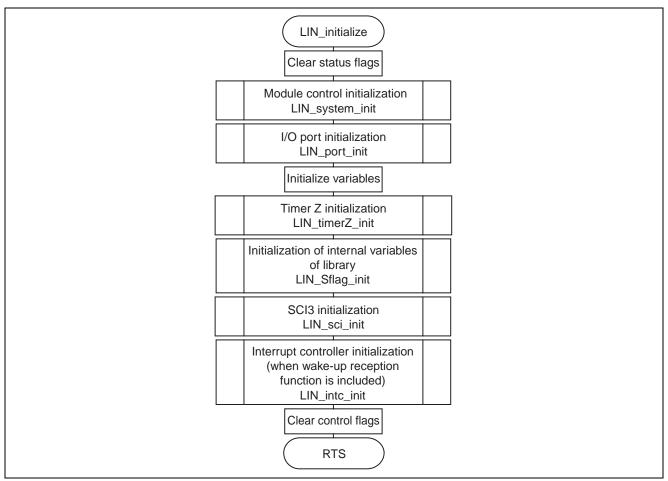
Figure 15 Initialization Function Flowchart
