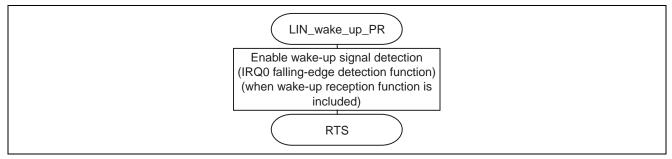
Figure 19 Flowchart of the Wake-up Signal Reception Preparation Function
