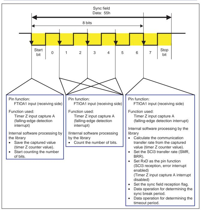
Figure 9 Correction of the Communication Transfer Rate by the Timer Z Input Capture Function
