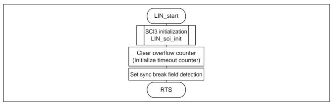
Figure 17 Flowchart of the LIN Communication Control Restart Preparation Functions
