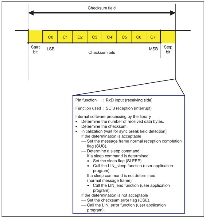
Figure 12 Checksum Field Reception and Determination
