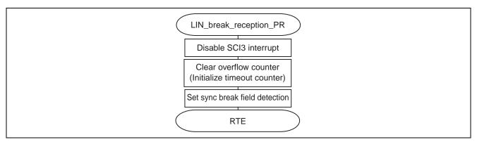
Figure 20 Function for Preparing for Sync Break Field Detection and Reception
