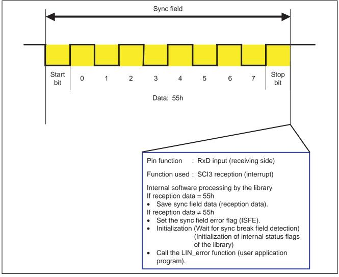
Figure 8 Reception and Determination of a Sync Field by the SCI3 Reception Function
