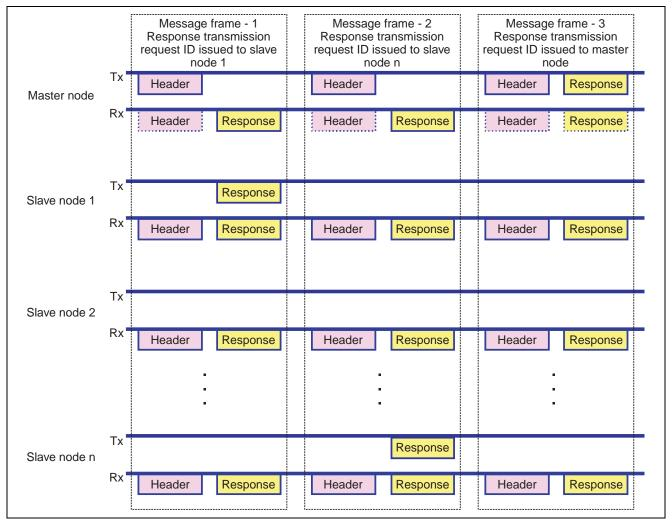
Figure 4 Transmission and Reception of Message Frames
