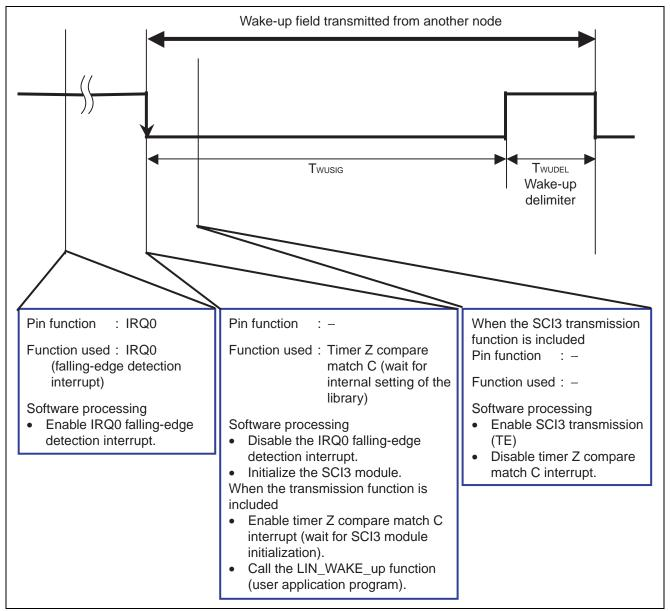
Figure 14 Reception of a Wake-up Signal
