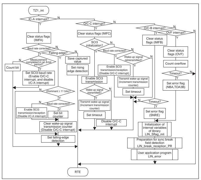
Figure 22 Flowchart of the Timer Z (channel-1) Interrupt Function
