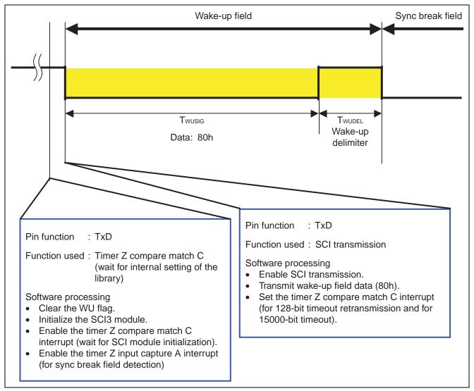
Figure 13 Transmission of a Wake-up Signal
