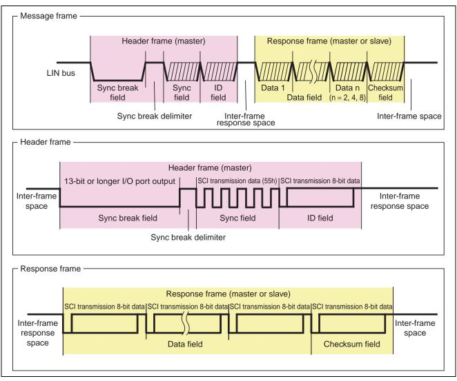
Figure 3 Message Frame Structure
