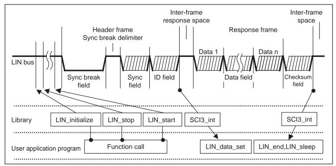
Figure 5 Operation Overview at Message Frame Transmission/Reception
