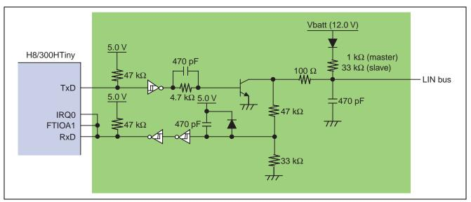
Figure 2 Sample LIN Bus Interface Circuit
