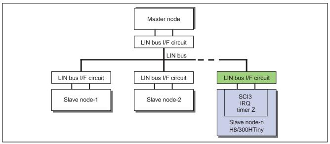
Figure 1 Block Diagram of a System Connected Through the LIN Bus
