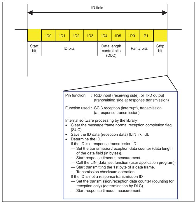
Figure 10 ID Field Reception and Determination
