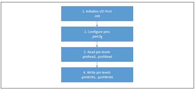
Figure 3 Flow Diagram of a Typical I/O Port HAL Module Application
