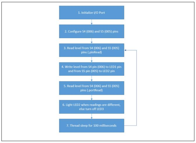
Figure 4 I/O Port HAL Module Application Project Flow Diagram
