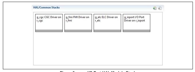
Figure 2 I/O Port HAL Module Stack
