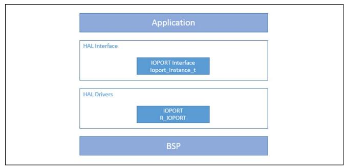
Figure 1 I/O Port HAL Module Block Diagram
