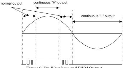
Figure 9. Sin Waveform and PWM Output
