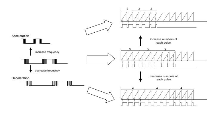
Figure 11. Changes of Stepping Motor Speed
