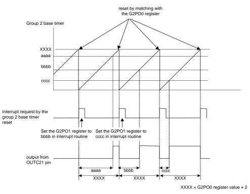
Figure 8. PWM Output Timing
