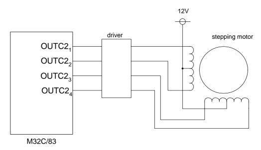
Figure 6. M32C/83 with Stepping Motor
