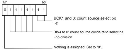
Supply to each register shown in procedures 6) to 13) and 20). To enable each register setting as soon as they are set, set the G2BCR0 register to "011111111b".
