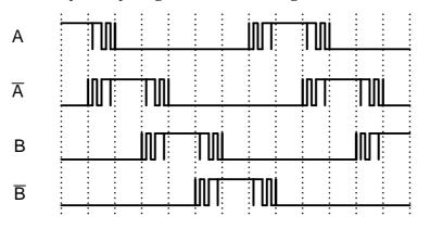
Figure 5. Microstepping Control (one-two excitation))
