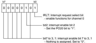
Set the interrupt request bit of unused interrupt to "0".
