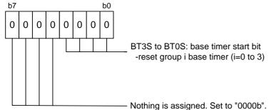
Clock is supplied to the BTSR register to enable the BTSR register setting.
