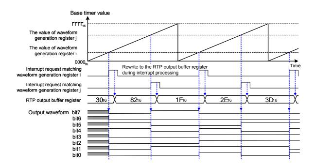
Figure 16 Parallel Real-Time Port Output Operation Timing Diagram
