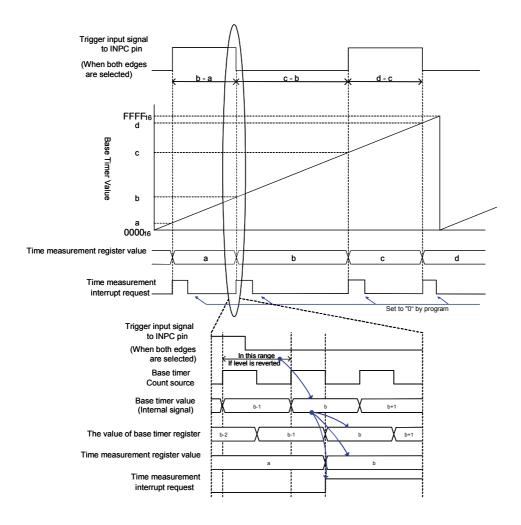
Figure 3 Input Capture Operation Diagram
