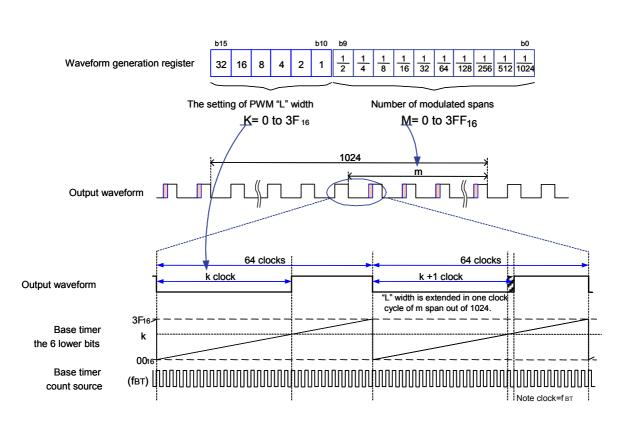
Figure 12 Bit Modulation PWM Output Schematic Drawing
