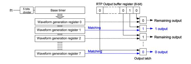
Figure 13 Configuration of Real-Time Port Output
