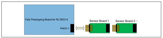
Figure 2-4 Hardware Connections for the RL78/G14 Group
