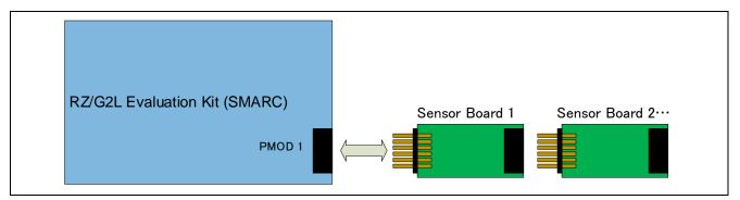
Figure 2-6 Hardware Connections for the RZ Family
