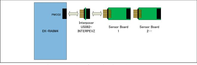
Figure 2-1 Hardware Connections for the RA6M4 Group
