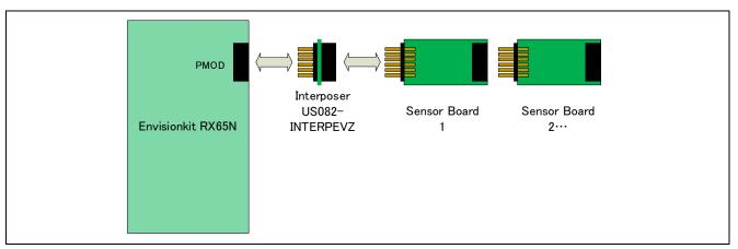
Figure 2-3 Hardware Connections for the RX Family
