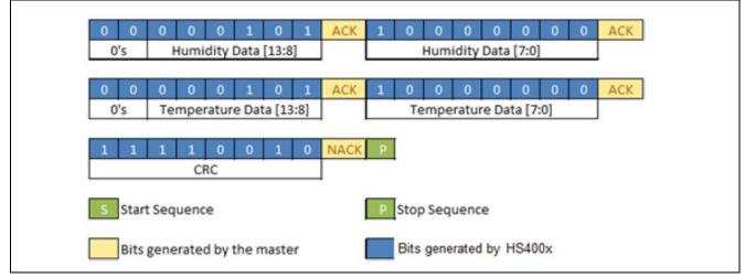
Figure 3-1 Format of I2C Communications
