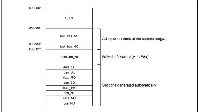
Figure 4.1 Application Example of Section Assignment
