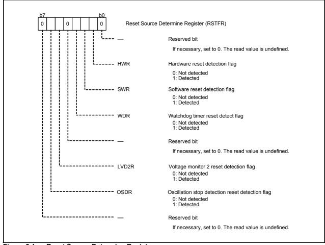
Figure 3.1 Reset Source Determine Register
