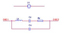
Figure 1.1 Equivalent Circuit
