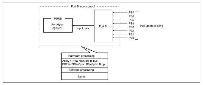
Figure 3.3 Processing for Open-Circuit Pins of Input Ports (e.g. Port B)
