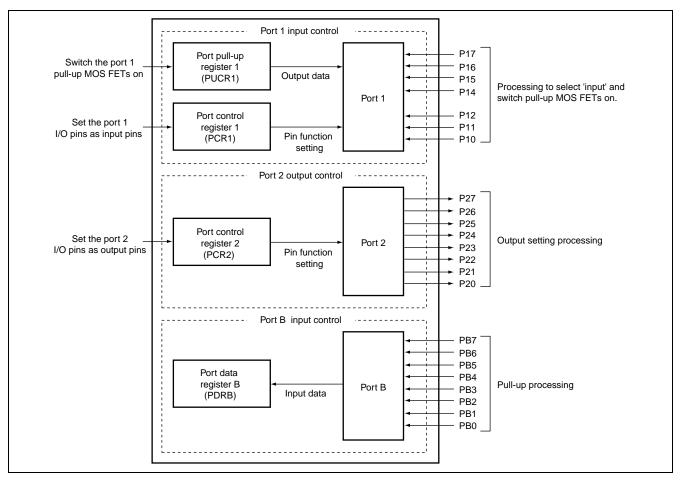
Figure 2.1 Settings for Open Pins on Ports 1, 2, and B
