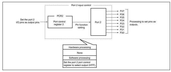
Figure 3.2 Processing for Open-Circuit Pins of General I/O Ports (e.g. Port 2)
