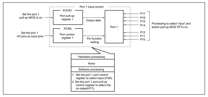
Figure 3.1 Processing for Open-Circuit Pins of Ports with Pull-Up MOSFETs (e.g. Port 1)
