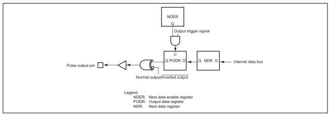
Figure 2 Schematic Diagram of PPG
