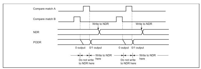
Figure 4 Non-Overlapping Operation and NDR Write Timing
