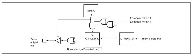
Figure 3 Non-Overlapping Pulse Output
