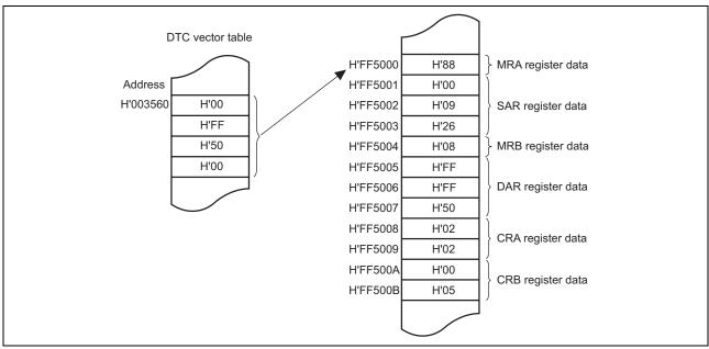
Figure 3 DTC Vector Table and Arrangement in Memory (Example of This Application Note)
