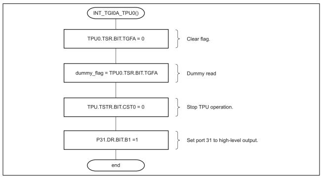
Figure 10 Flowchart (DTC End Interrupt)
