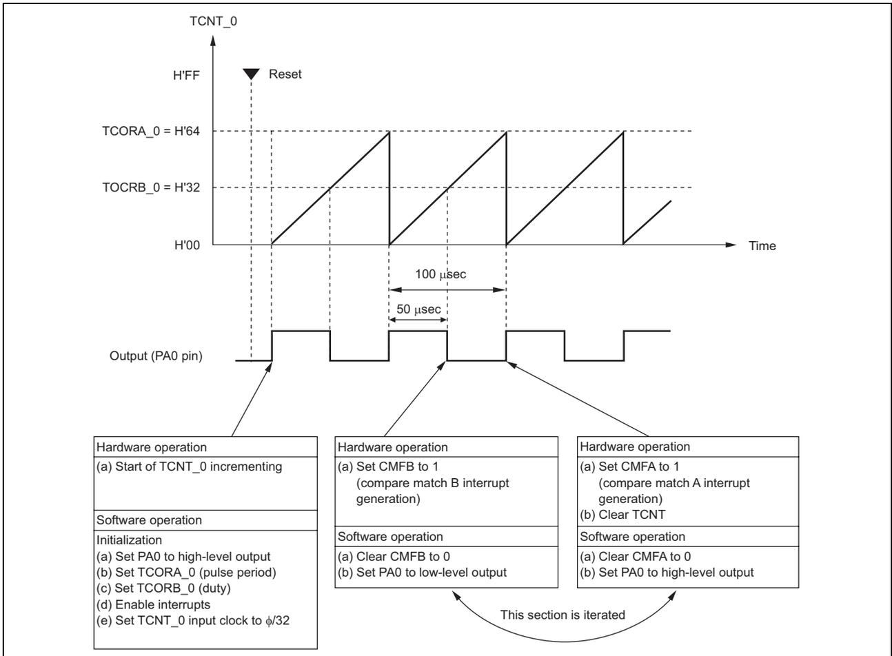
Figure 5 8-Bit Timer (TMR) Pulse Signal Generation
