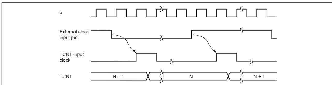
Figure 2 Count Timing for Internal Clock Input
