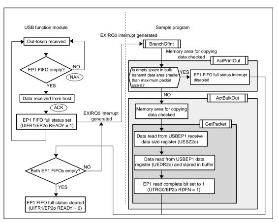
The operation of the sample program in bulk-out transfers is shown in figure 5.15.
