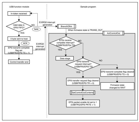
Figure 5.13 Status Stage (Control-Out Transfer)
