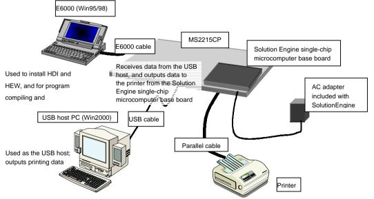
Figure 3.1 Device Connections
