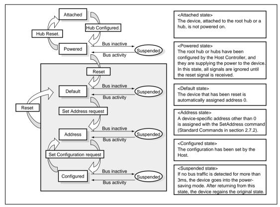
Figure 2.25 USB Device State
