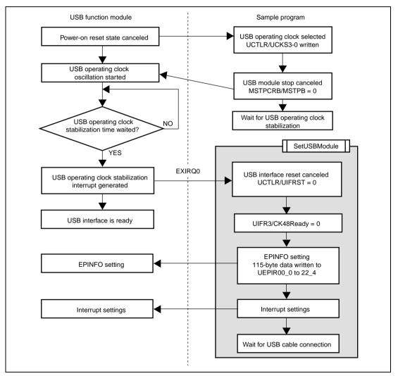
Figure 5.3 USB Operating Clock Stabilization Interrupt
