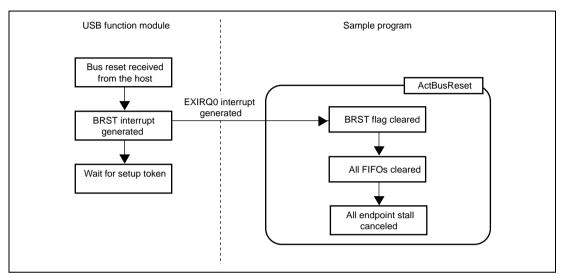
Figure 5.6 Bus Reset Interrupt
