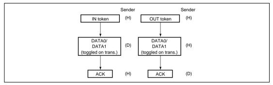
Figure 2.19 Data stage (left: IN, right: OUT)
