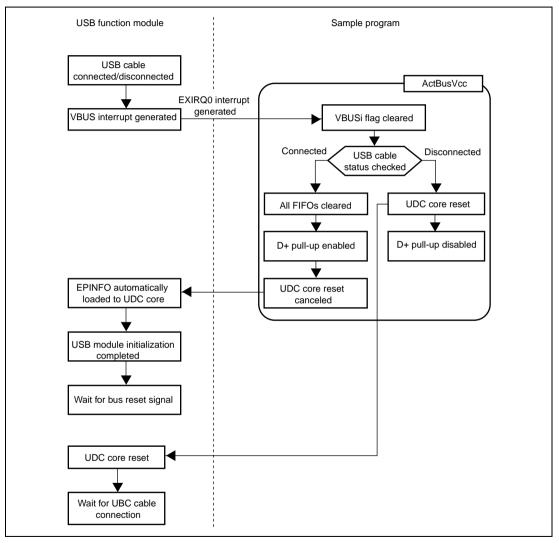
Figure 5.5 Interrupt on Cable Connection
