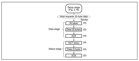
Figure 2.21 Data Stage Interrupted
