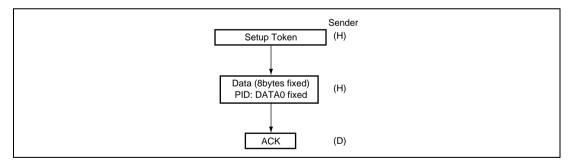
Figure 2.18 Setup Stage
