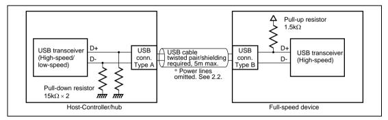
Figure 2.8 For Full-Speed Devices
