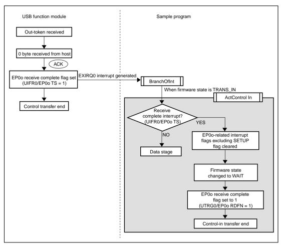
Figure 5.12 Status Stage (Control-In Transfer)
