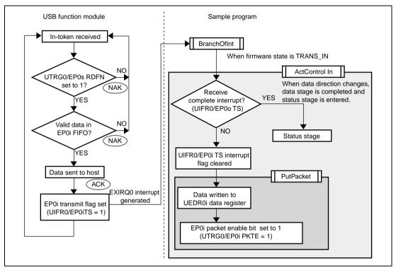
Figure 5.10 Data Stage (Control-In Transfer)
