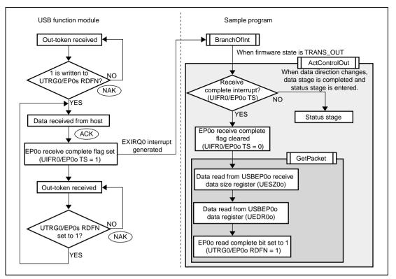
Figure 5.11 Data Stage (Control-Out Transfer)
