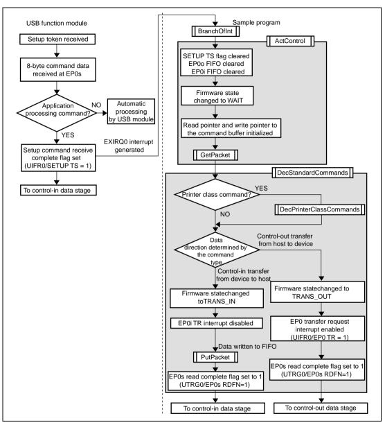
Figure 5.9 Setup Stage
