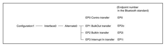
Figure 5.4 Endpoint Configuration in the Sample Program
