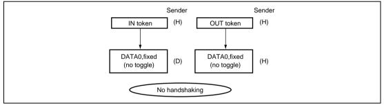
Figure 2.23 Isochronous Transfer (left: IN, right: OUT)
