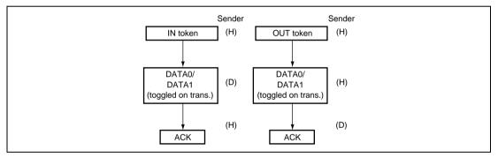
Figure 2.22 Bulk Transfer (left: IN, right: OUT)
