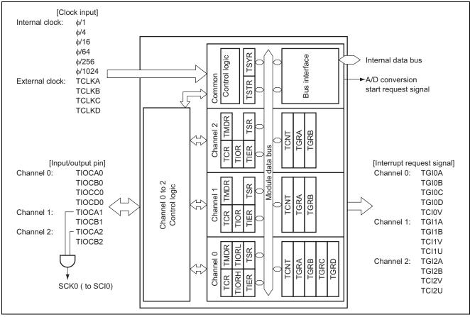
Figure 2.1 Block Diagram of TPU
