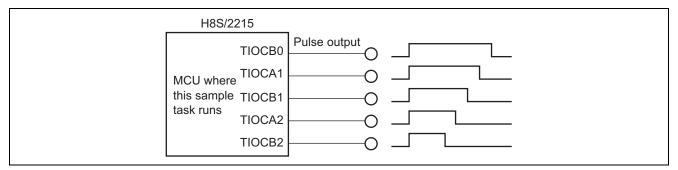
Figure 1.1 Example of PWM Pulse Output
