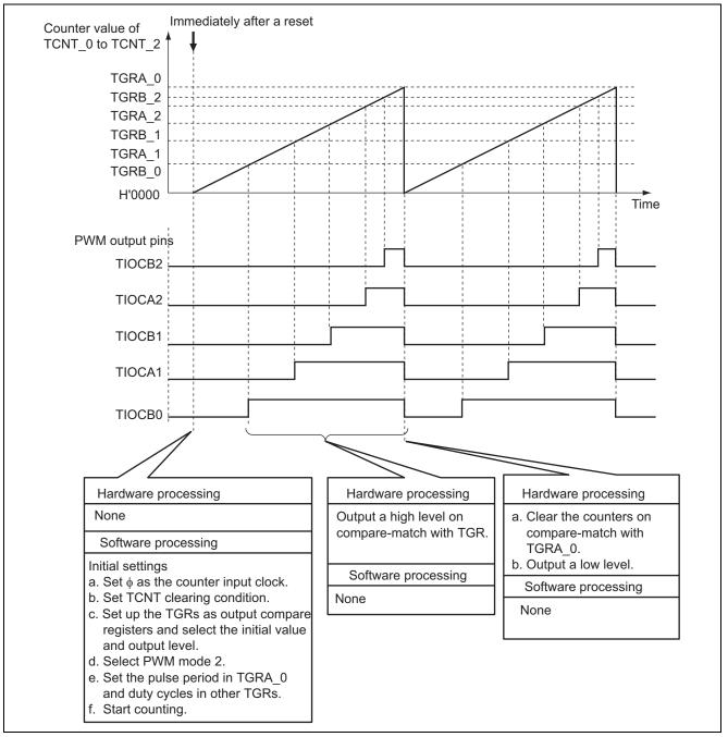
Figure 3 PWM Pulse Output Operation
