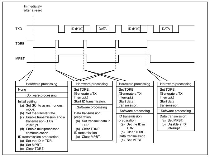
Figure 4 Principles of Operations Used for Multiprocessor Communication (Transmitting Station)
