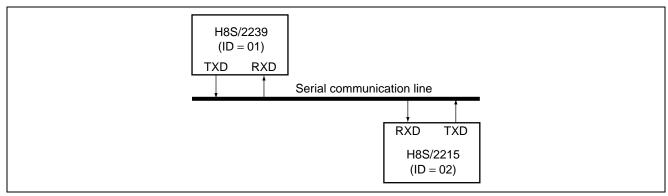
Figure 1 Block Diagram of Asynchronous SCI Using Multiprocessor Function
