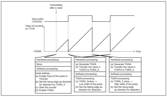
Figure 3 Measuring the Pulse Width
