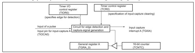
Figure 2 Blocks Used in Measuring the High and Low Periods of a Pulse
